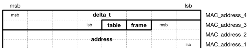
Figure 20: Mapping of real time parameters in MAC_address field
