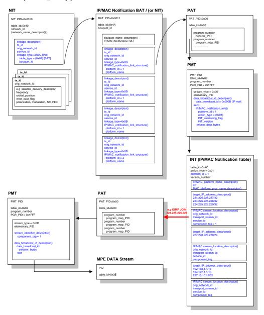
Figure 3: Example for IP/MAC streams with INT reference
