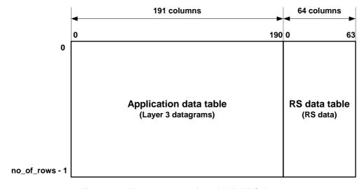
Figure 13: The structure of the MPE-FEC Frame
