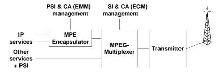
Figure 11: Headend construction for mixed multiplex
