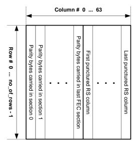
Figure 16: The layout of the RS data table
