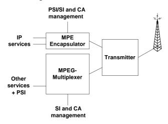
Figure 12: Headend construction for hierarchical transmission
