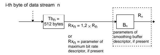
Figure 23: Data service decoder model
