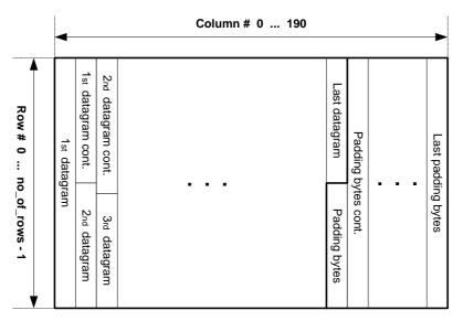
Figure 15: The layout of the Application data table
