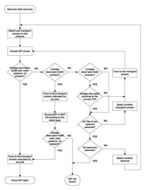
Figure 2: Example procedure to locate IP/MAC Notification Table for a receiver which knows, in advance, the platform\_id
