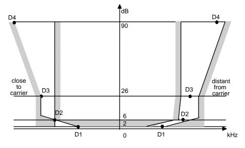
Figure B.2: IF filter characteristics
