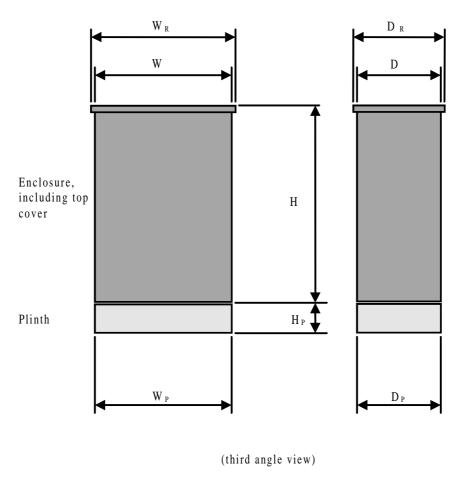
Figure A.1: Co-ordination dimensions of outdoor enclosures/basic views
