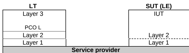
Figure 1: Remote test method
