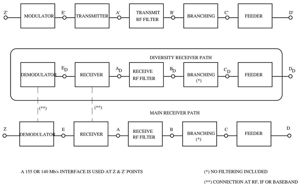
Figure 1: Block Diagram
