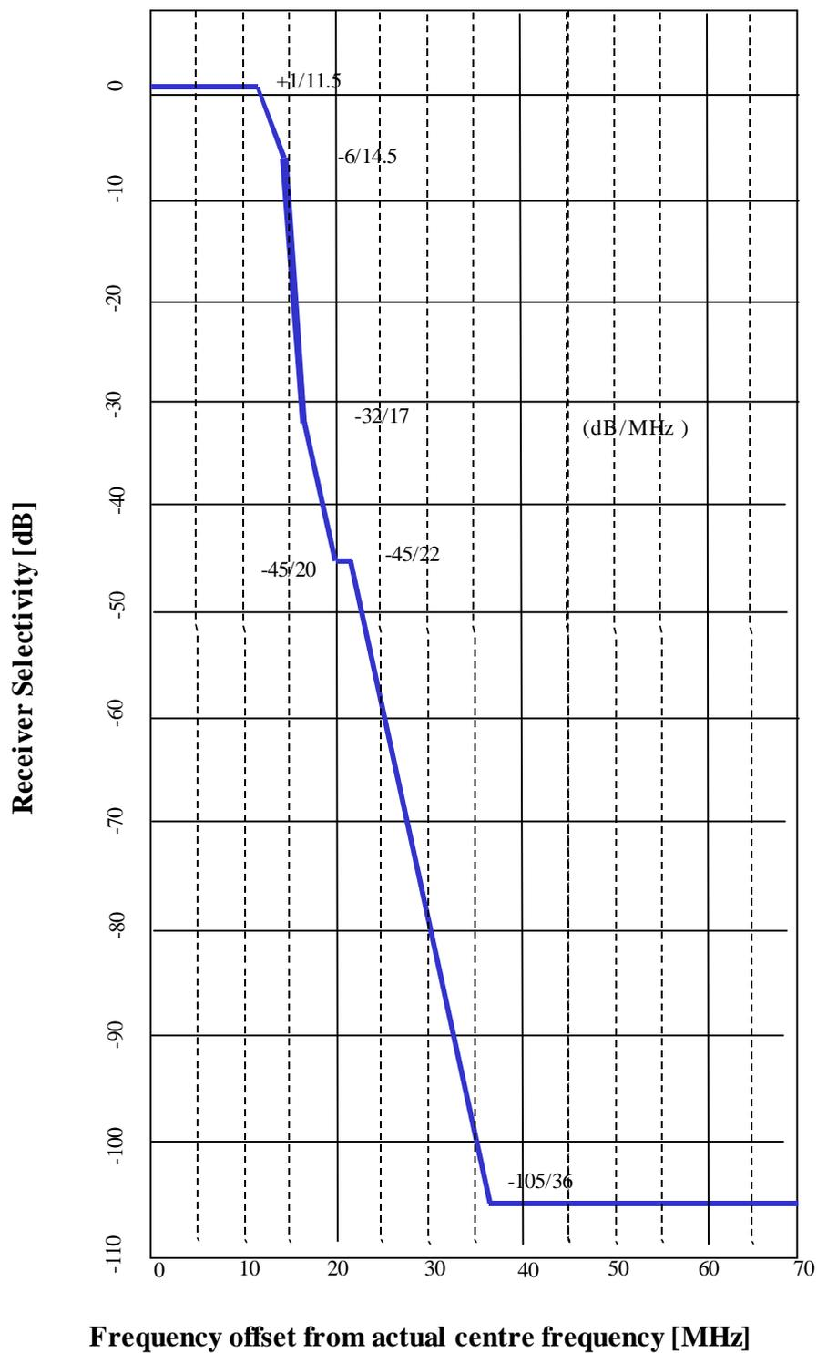
Figure 4: Limits for the receiver selectivity for the inner edges of the innermost channels in the 6L GHz band
