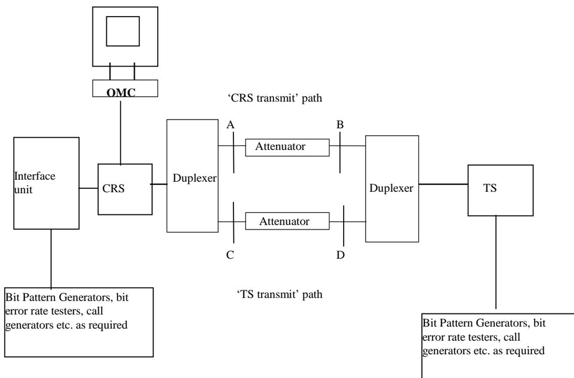
Figure 3: Test configuration for a single Terminal Station
