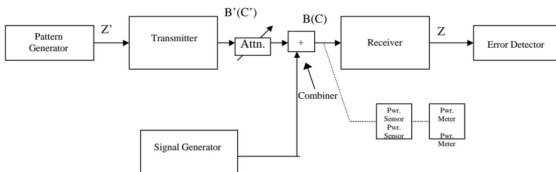
**Figure 15: Test configuration for CW spurious interference**Test Procedure:
