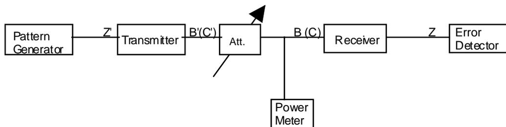
**Figure 14: Test configuration for background BER**
