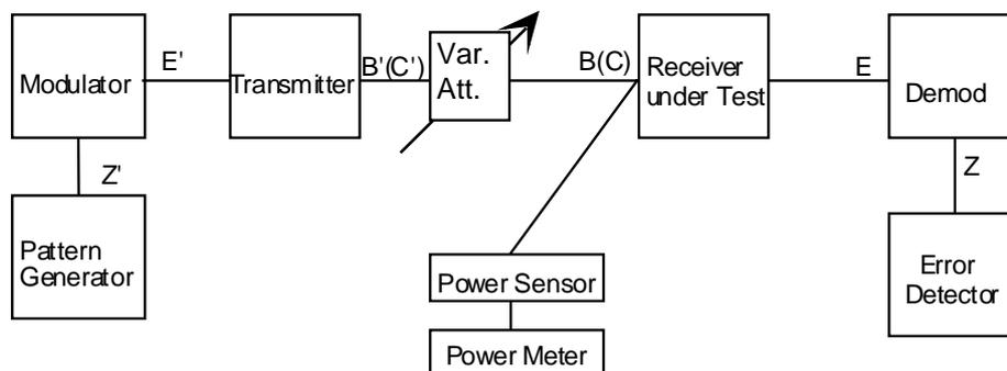
**Figure 11: Test configuration for input level range**
