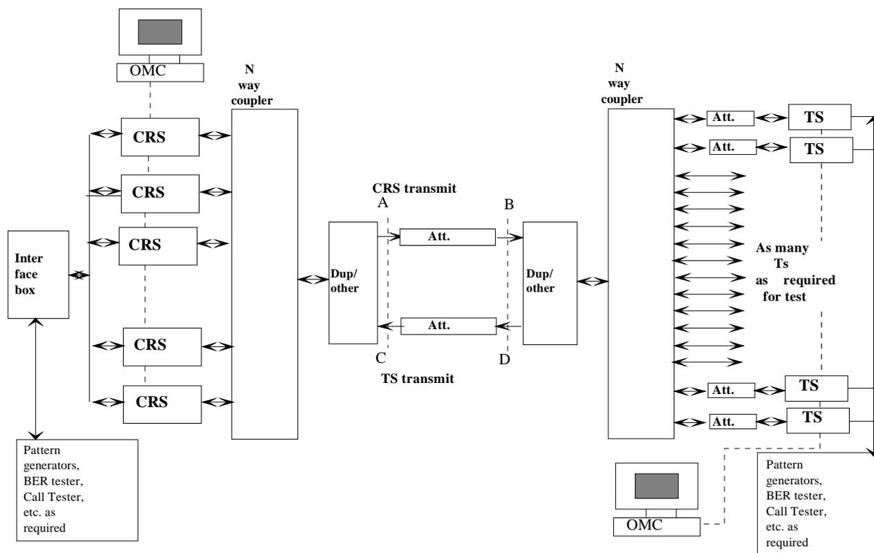
**Figure 5: Test Configuration for multiple CRS and TS**
