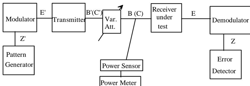
**Figure 9: Test Configuration for input level range**
