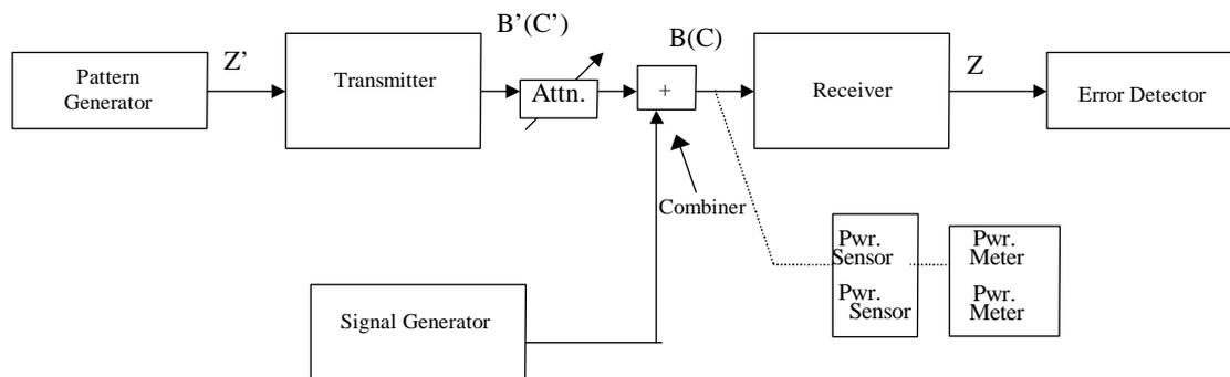
**Figure 14: Test configuration for CW spurious interference**
