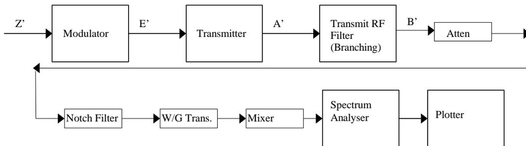
**Figure 8: Test Configuration for conducted antenna port spurious emissions**
