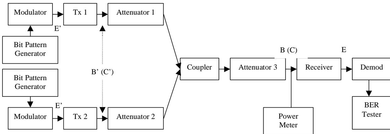
**Figure 13: Test configuration for Co-channel Interference Sensitivity - external**
