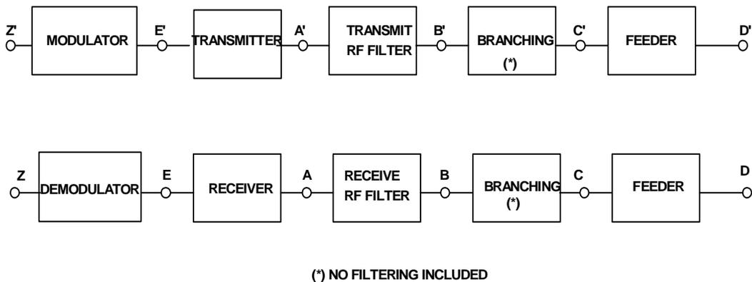
Figure 2: RF System Block diagram
