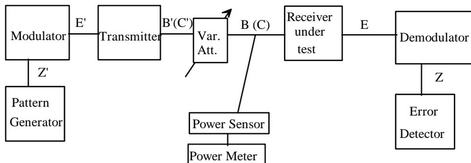
**Figure 10: Test configuration for dynamic level range**
