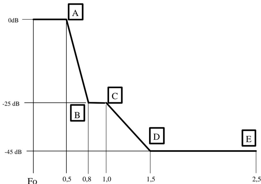
Figure 3: DS-CDMA spectrum mask normalized for channel spacing
