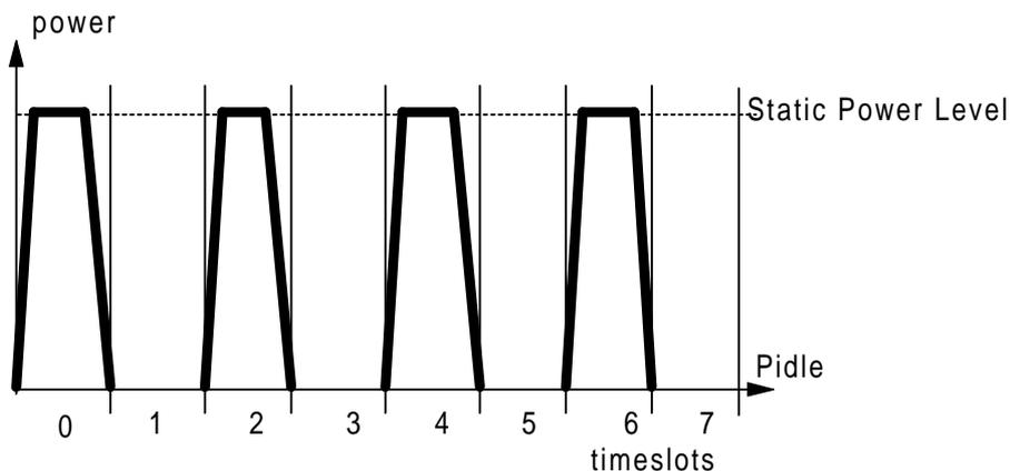
Figure 4: Power/time slot configuration (no RF power control)
