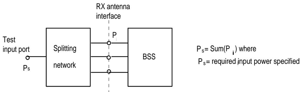
**Figure 1a: Receiver test setup**
