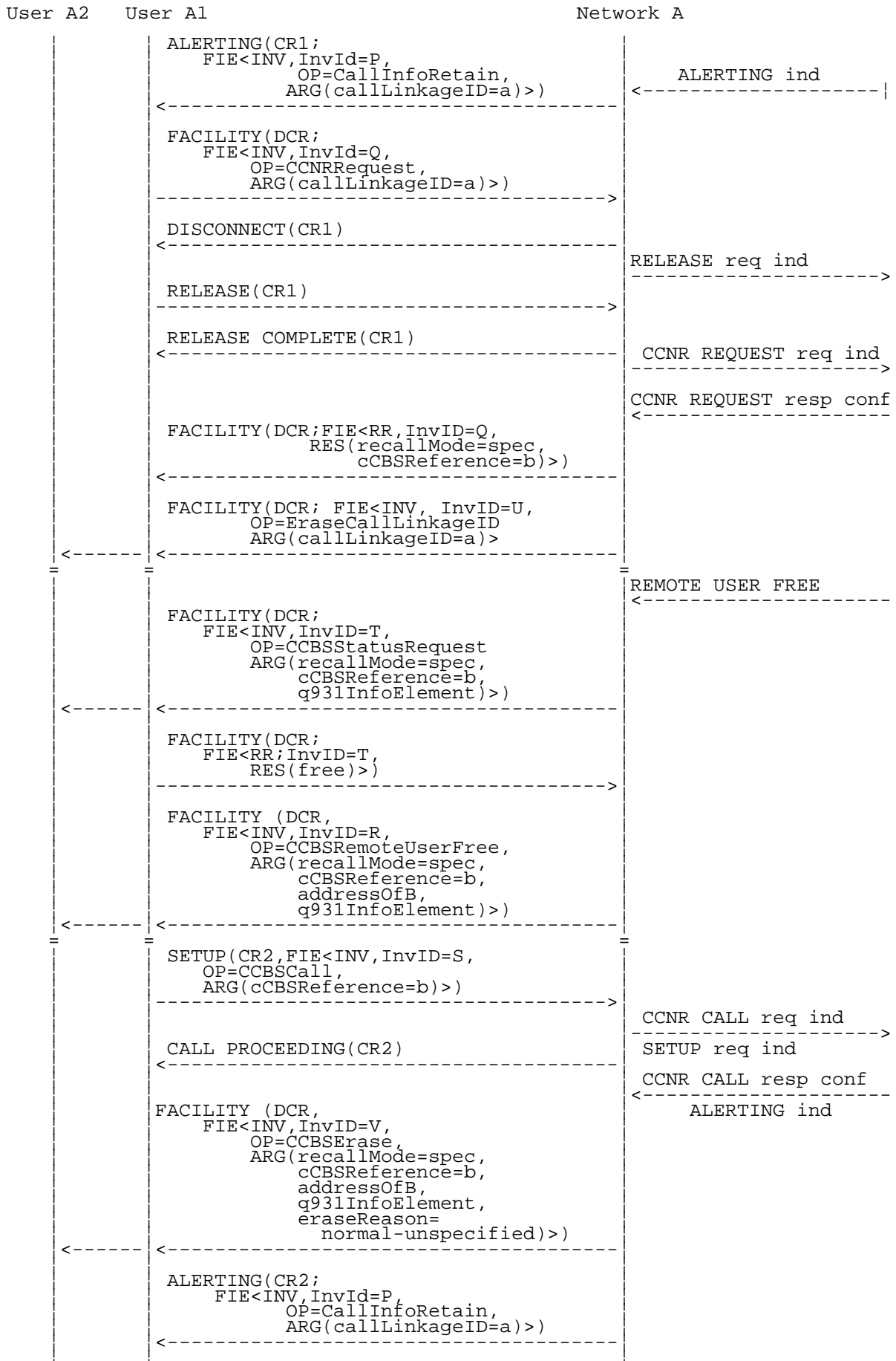
Figure A.1: Normal operation, CCNR request during the alerting phase, "CCBS request retention" option is set to "no", specific recall, user A free
