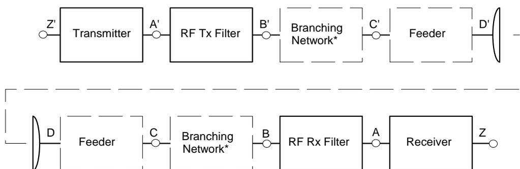
NOTE: Points B & C and B' and C' will coincide if branching networks are not used.
