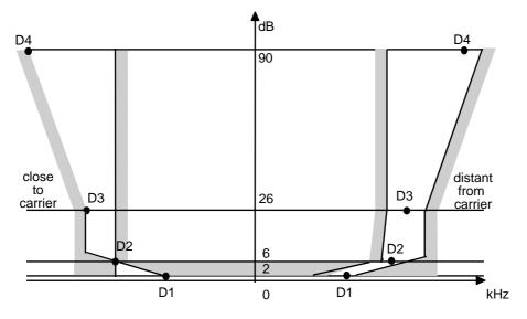
Figure B.1: IF filter characteristics
