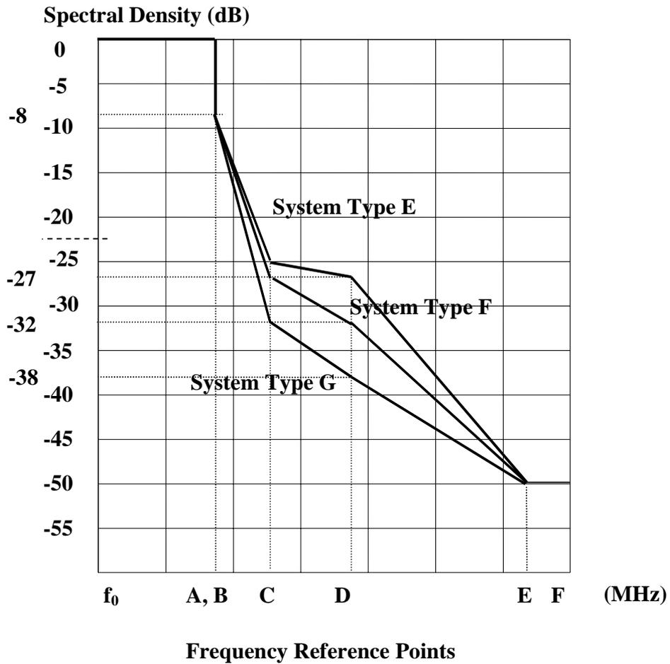
Figure 4: Power spectrum masks for system type E, F and G ( $f_0$  = actual carrier frequency)
