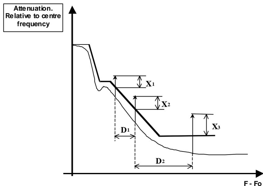
$$X_1, X_2, X_3 \text{ [dB]} \leq 10\log(\text{CSmin}/\text{IFbw})-10$$
