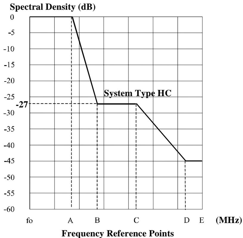
Figure 5: Power spectrum masks for system type HC ( $f_0$  = actual carrier frequency)
