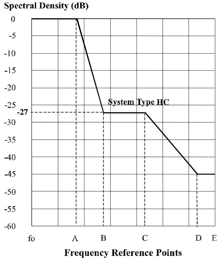
**Figure 5: Power spectrum masks for system type HC ( $f_o$  = actual carrier frequency)**
