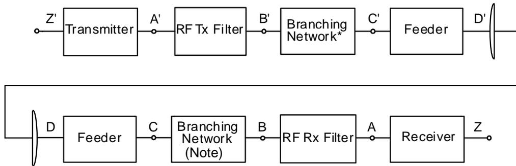
NOTE: Points B and C and B' and C' will coincide if branching networks are not used.
