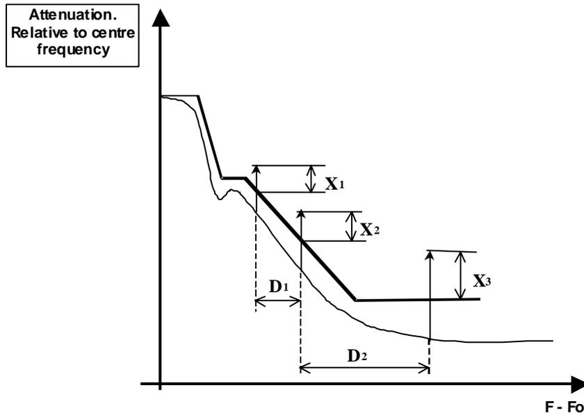
$$X_1, X_2, X_3 \text{ [dB]} \leq 10\log(\text{CSmin}/\text{IFbw})-10$$
