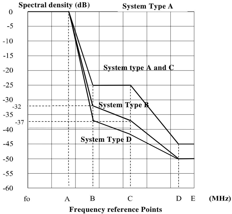
Figure 3: Power spectrum masks for system type A, B, C and D ( $f_0$  = actual carrier frequency)
