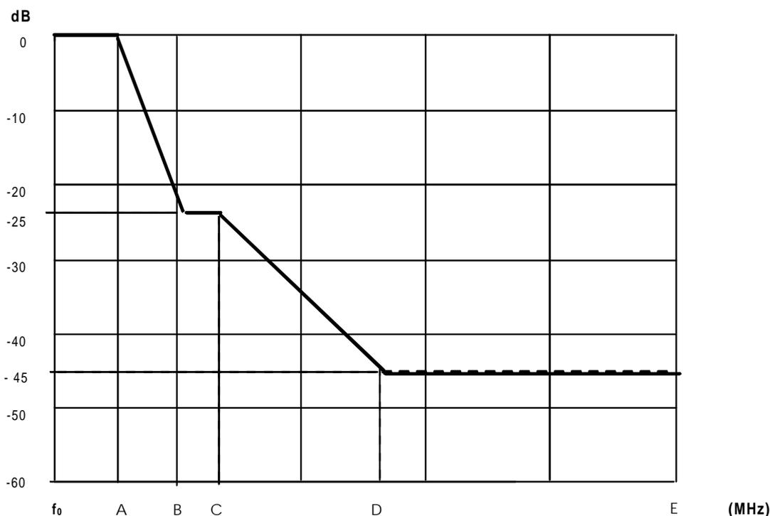
Figure 3: Power spectrum mask ( $f_0$  = actual carrier frequency)
