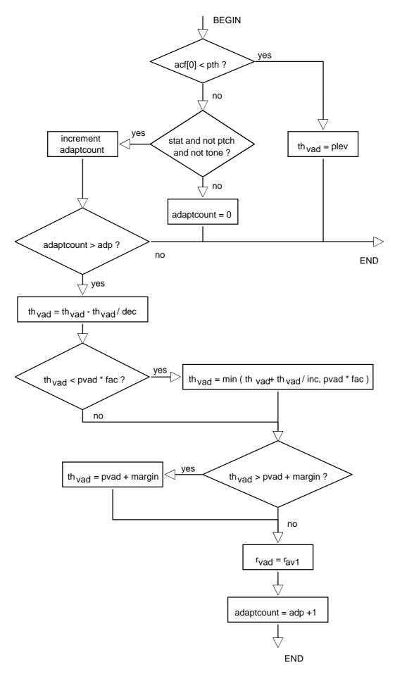
Figure 2: Flow diagram for threshold adaptation
