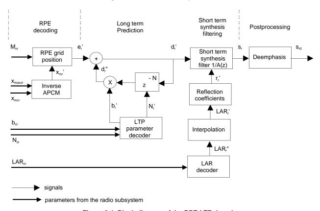
Figure 3.4: Block diagram of the RPE-LTP decoder
