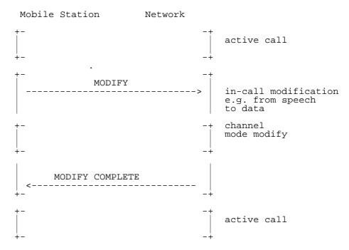
Figure 7.17/GSM 04.08: In-call modification
