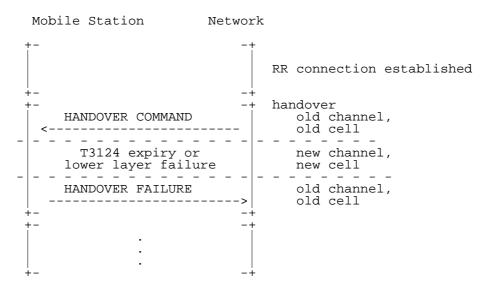
Figure 7.16/GSM 04.08: Handover failure, reconnection to the old traffic channel
