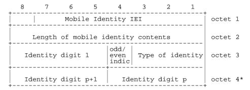
Figure 10.5.4/GSM 04.08: Mobile Identity information element
