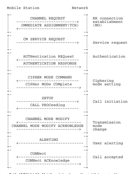
Figure 7.10c/GSM 04.08: Mobile originating call establishment with very early assignment
