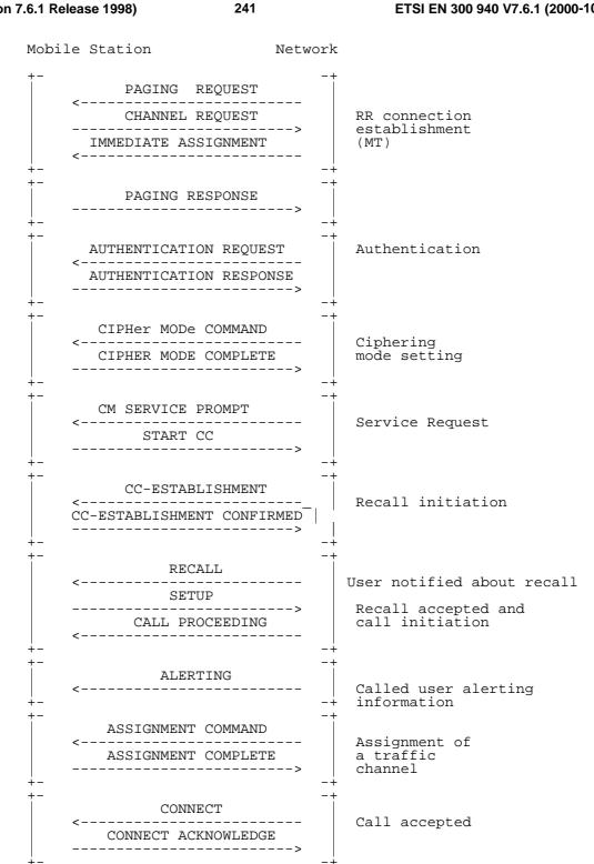
Figure 7.21/GSM 04.08: Network initiated mobile originating call establishment with assignment after A and B party alerting
