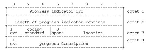
Figure 10.5.107/GSM 04.08: Progress indicator information element
