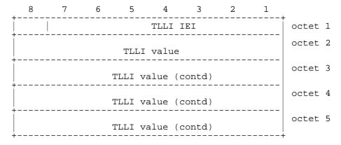
Figure 10.5.69/GSM 04.08: TLLI information element
