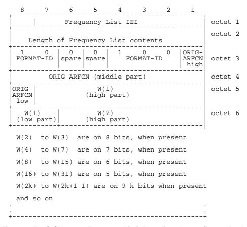
Figure 10.5.37/GSM 04.08: Frequency List information element (Range 512 format)
