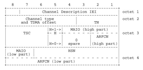
Figure 10.5.25/GSM 04.08: Channel Description information element
