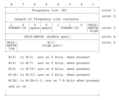
Figure 10.5.39/GSM 04.08: Frequency List information element (Range 128 format)
