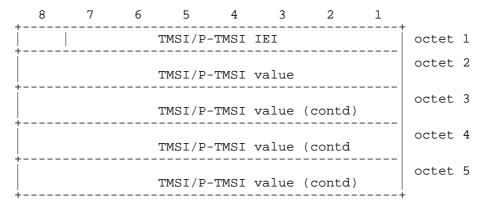
Figure 10.5.70/GSM 04.08: TMSI/P-TMSI information element
