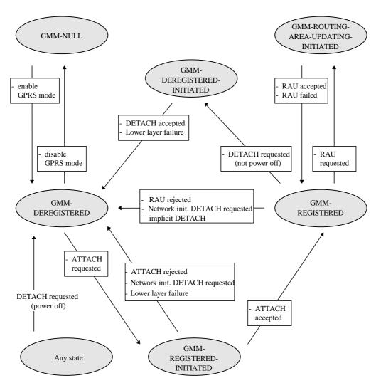
Figure 4.1b/GSM 04.08:GMM main states in the MS
