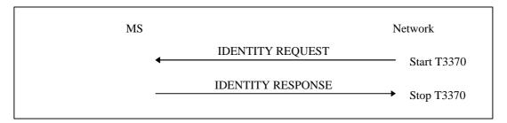
Figure 4.7.8/1 GSM 04.08: Identification procedure
