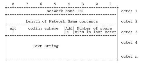
Figure 10.5.80/GSM 04.08: Network Name information element
