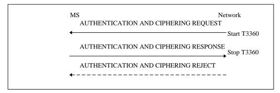
Figure 4.7.7/1 GSM 04.08: Authentication and ciphering procedure
