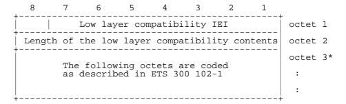
Figure 10.5.104/GSM 04.08: Low layer compatibility information element
