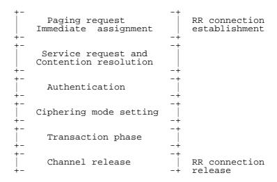
Figure 7.1/GSM 04.08: Components of structured procedures
