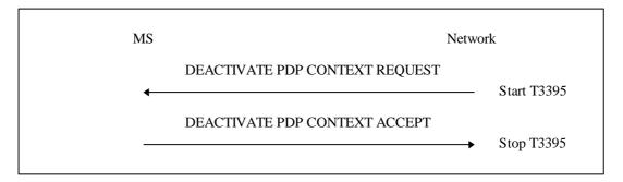
Figure 6.7/GSM 04.08: Network initiated PDP context deactivation procedure
