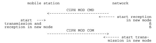
Figure 3.3/GSM 04.08: Ciphering mode setting sequence
