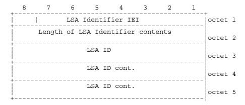
Figure 10.68c/GSM 04.08: LSA Identifier information element
