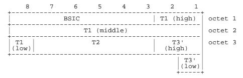
Figure 9.3/GSM 04.08: Frame synchronization information element
