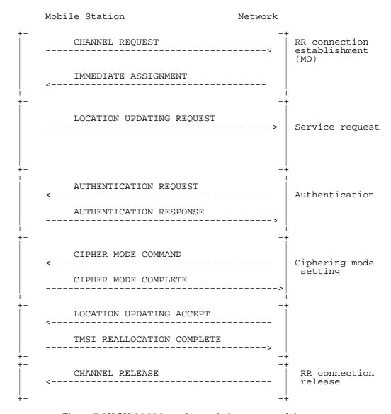
Figure 7.9/GSM 04.08 Location updating: successful case
