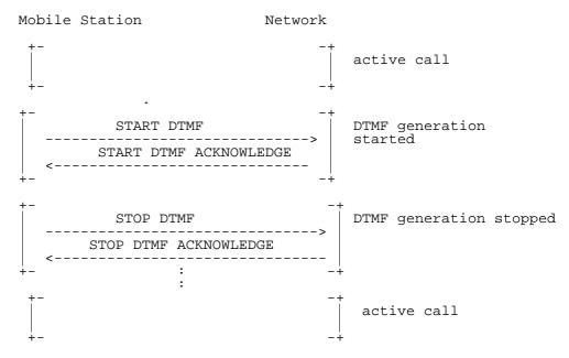
Figure 7.13/GSM 04.08: DTMF protocol control
