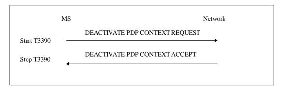
Figure 6.6/GSM 04.08: MS initiated PDP context deactivation procedure
