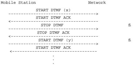
Figure 5.9/GSM 04.08: Multiple DTMF transmission
