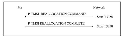
Figure 4.7.6/1 GSM 04.08: P-TMSI reallocation procedure
