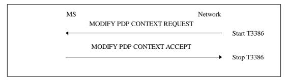
Figure 6.5/GSM 04.08: PDP context modification procedure
