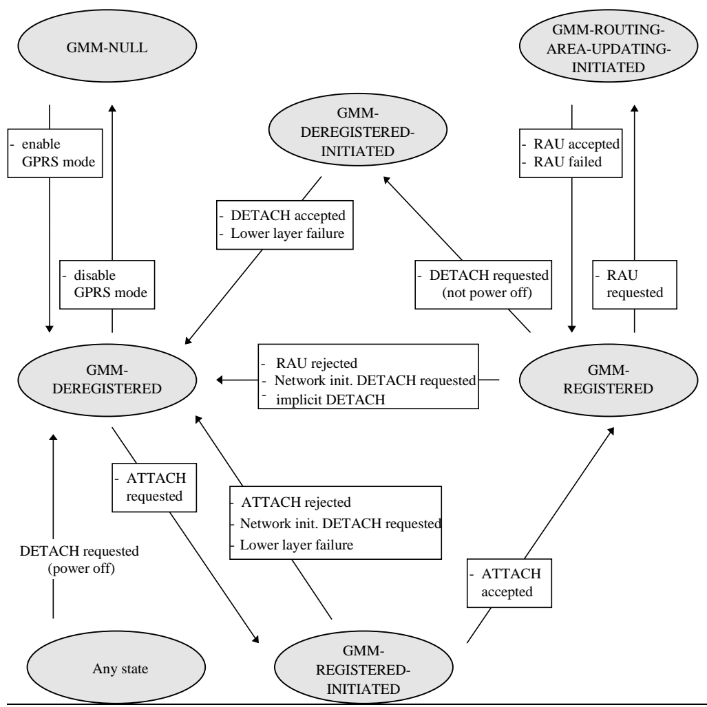
Figure 4.1b/GSM 04.08: GMM main states in the MS
