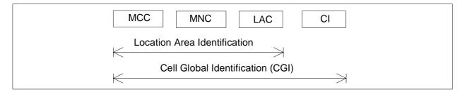
Figure 4: Structure of Cell Global Identification
