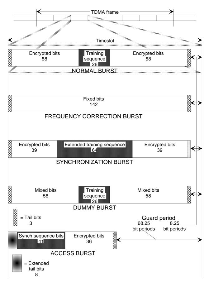
Figure 3: Timeslot and format of bursts
