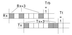
There is no requirement for relative timing of Tx timeslots in relation to Rx timeslots
