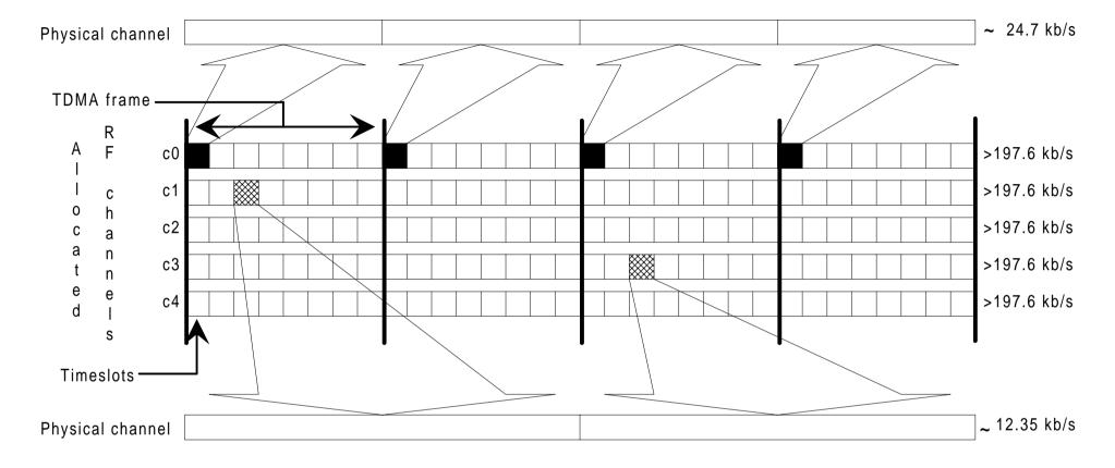
(This example of a physical channel is hopping using 3 of every other TDMA frame)
