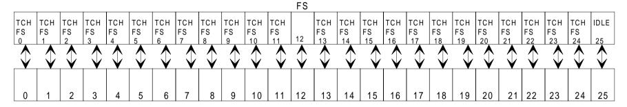
Figure 7a: TDMA frame mapping for TCH/FS + SACCH/FS
