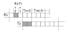
Alternative uplink biased assymetry (not prohibited by multislot class)
