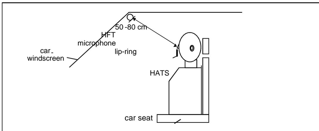
Figure 10: Measurement configuration for car type applications
