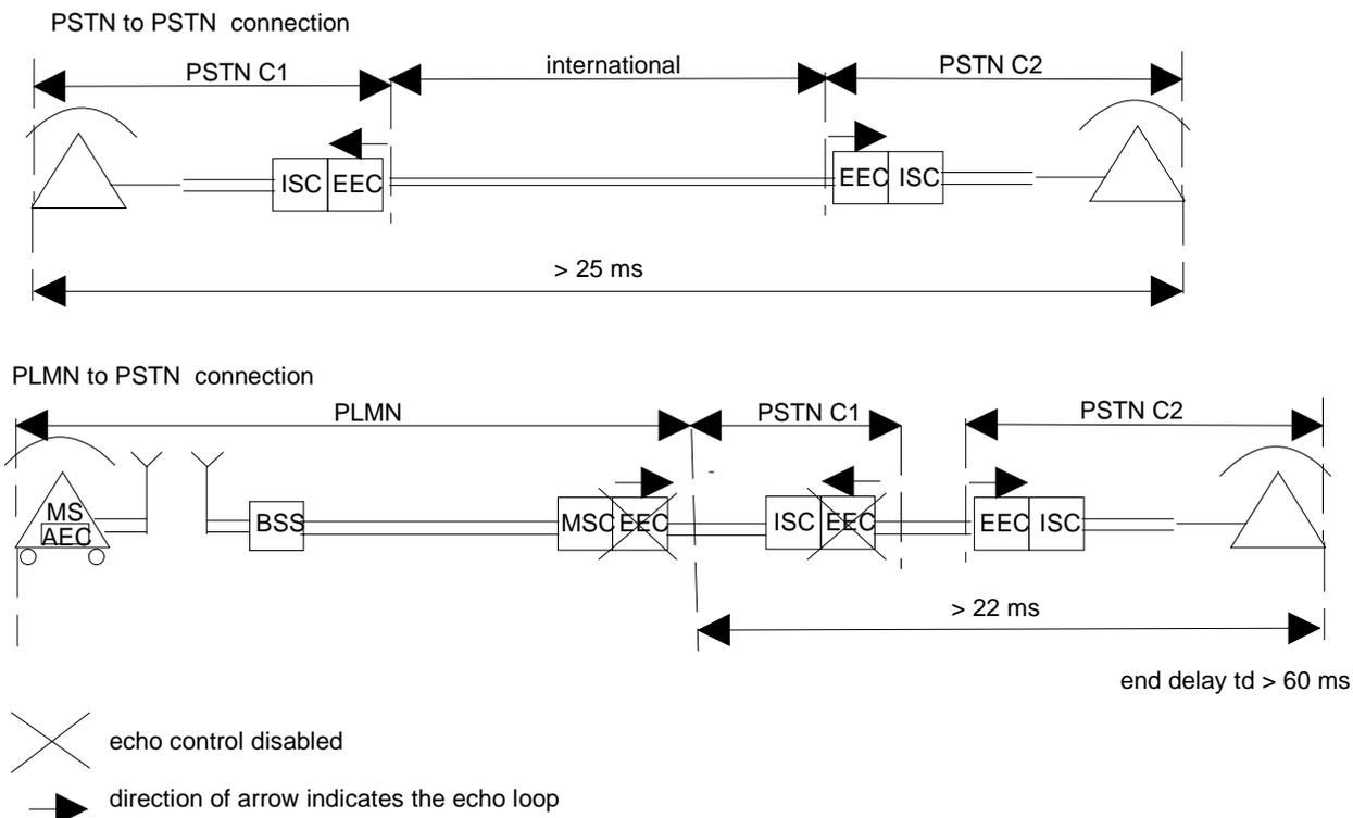
Figure 7: End Delay Requirements for PLMN EEC
