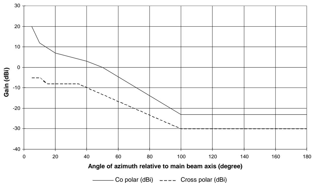
Figure 4c): RPEs for class 3 antennas in the frequency range 3
