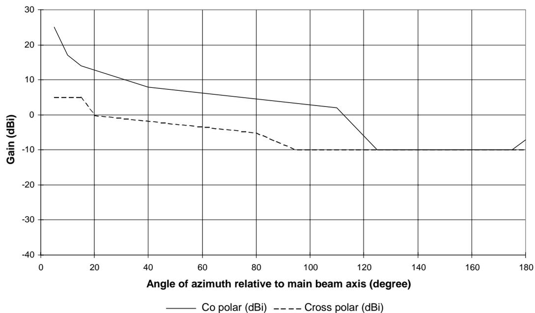
Figure 6a): RPEs for class 1 antennas in the frequency range 5
