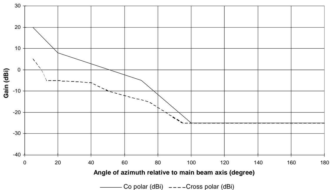
Figure 2c): RPEs for class 3 antennas in the frequency range 1
