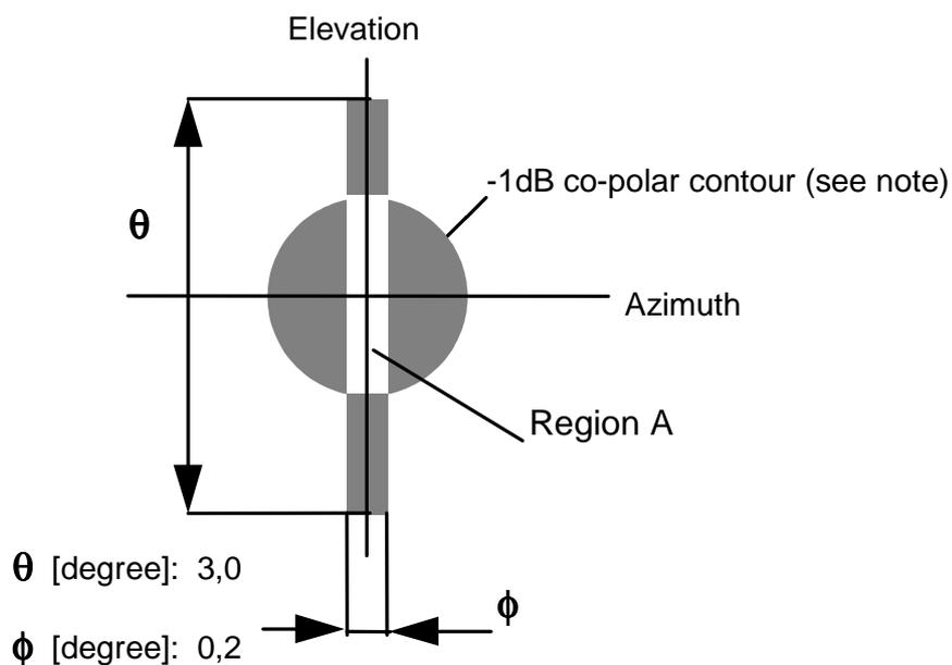
NOTE: For the dual band antennas -1 dB contour for highest frequency band shall be used.
