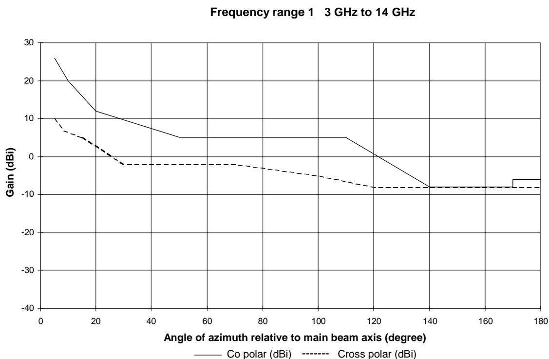
**Figure 2a): RPEs for class 1 antennas in the frequency range 1**
