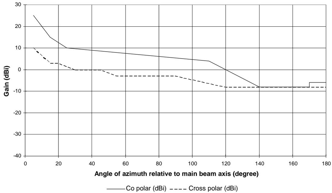
Figure 3a): RPEs for class 1 antennas in the frequency range 2
