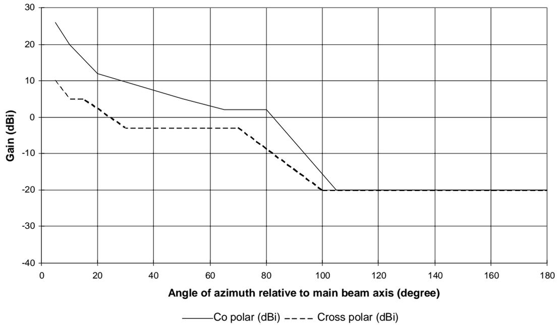
Figure 2b): RPEs for class 2 antennas in the frequency range 1
