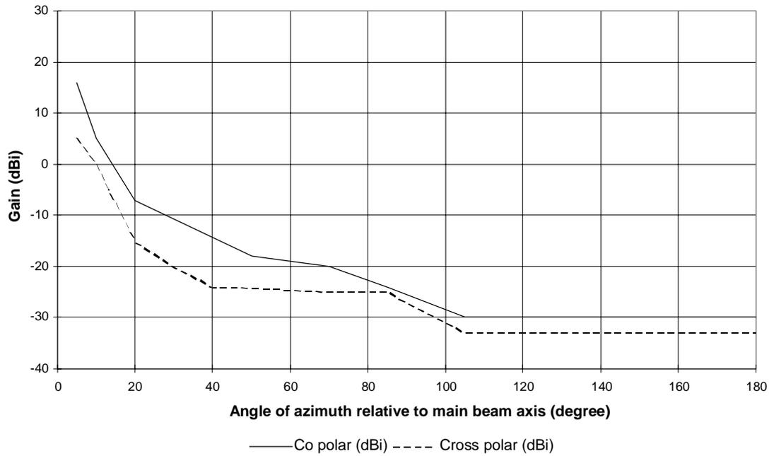
Figure 2d): RPEs for class 4 antennas in the frequency range 1
