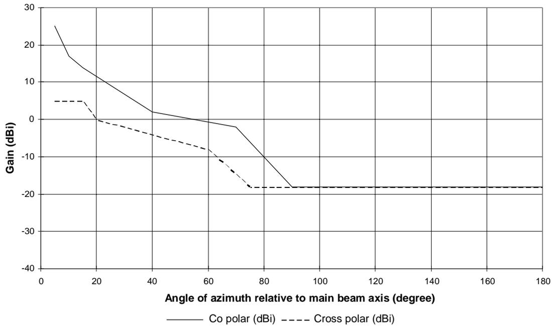
Figure 7b): RPEs for class 2 antennas in the frequency range 6
