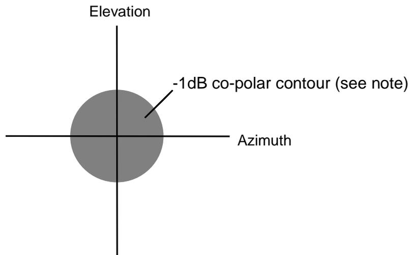
NOTE: For the dual band antennas -1 dB contour for highest frequency band shall be used.
