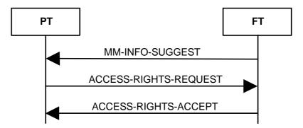
Figure 3: On air modification of user parameters
