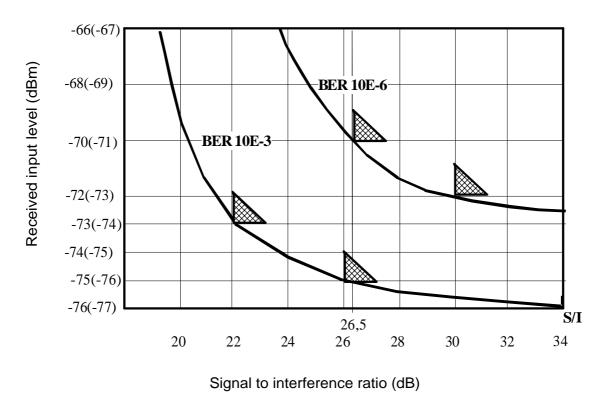
NOTE: Values for received input level refer to the 15 GHz and 18 GHz bands, values in brackets refer to 13 GHz band.
