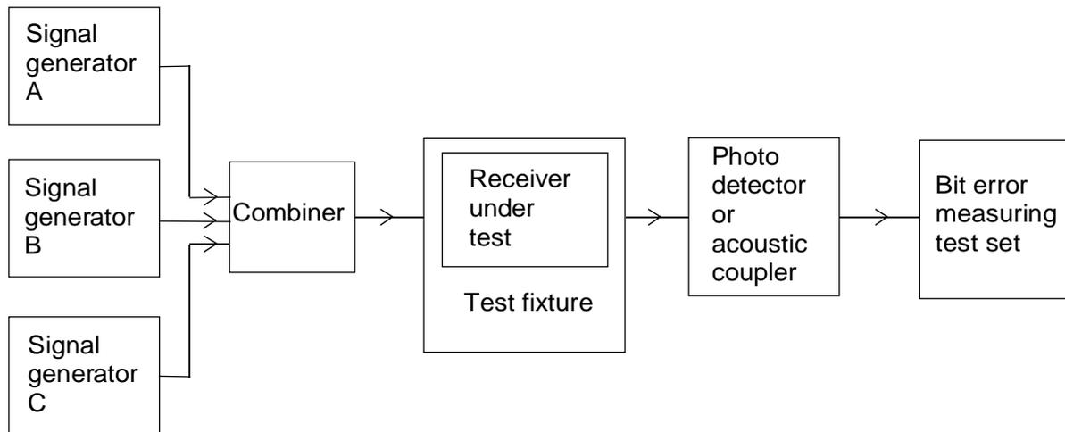
**Figure 10: Measurement arrangement - intermodulation response rejection**
