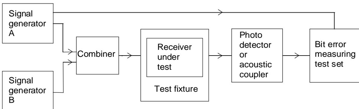
**Figure 9: Measurement arrangement - spurious response rejection**
