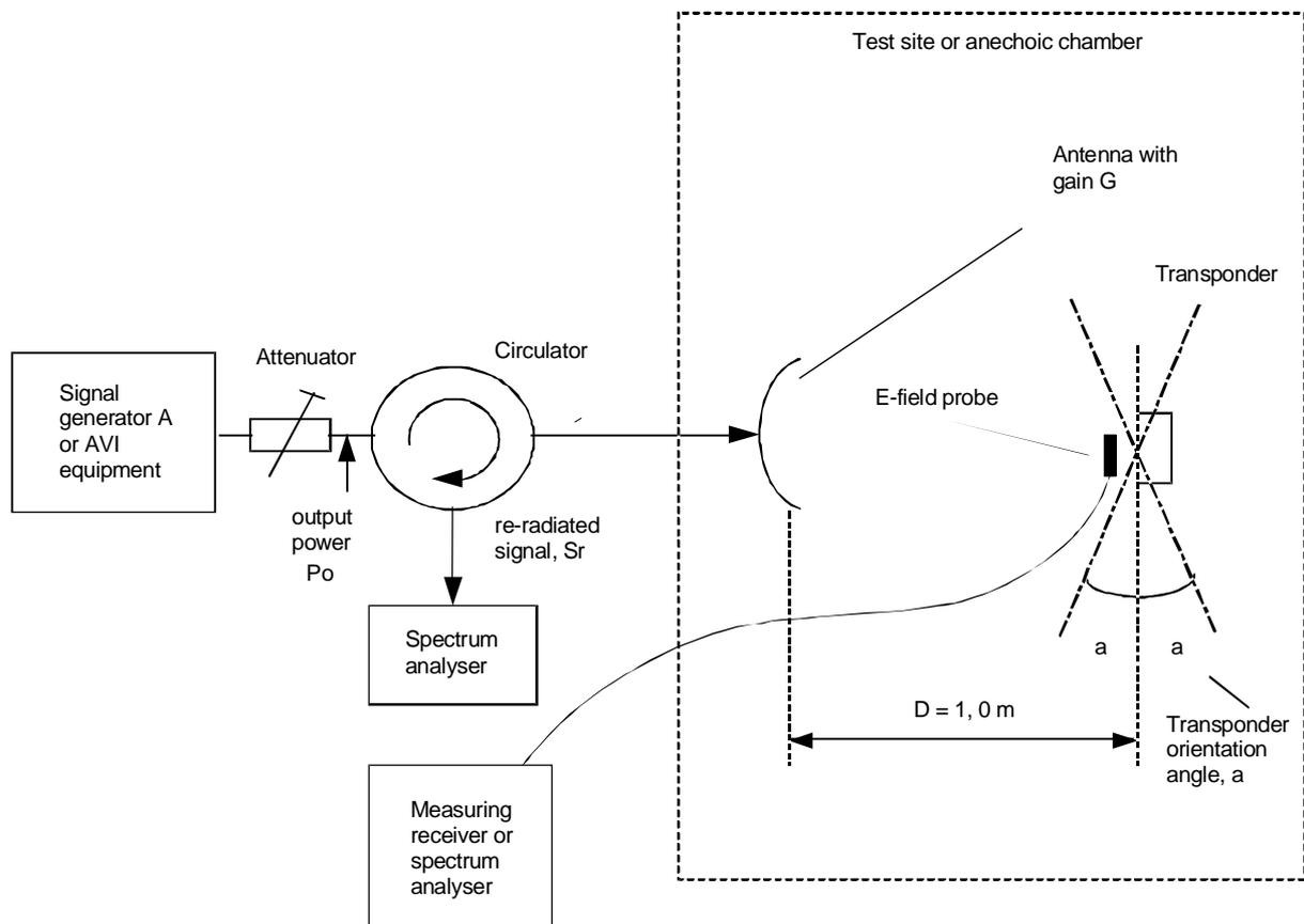
**Figure 12: Test arrangement - transponder wake up**
