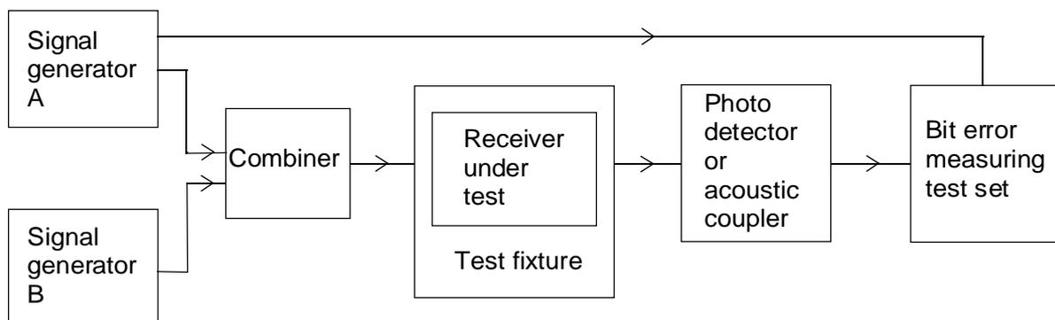
**Figure 8: Measurement arrangement - adjacent channel selectivity**
