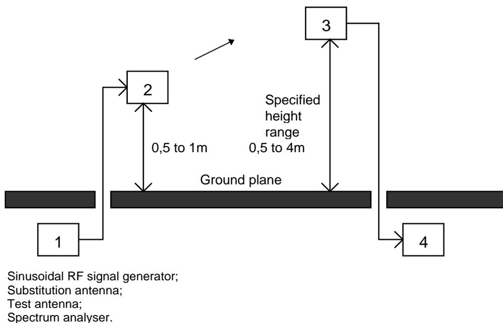
**Figure C.2: Measurement arrangement No. 2**
