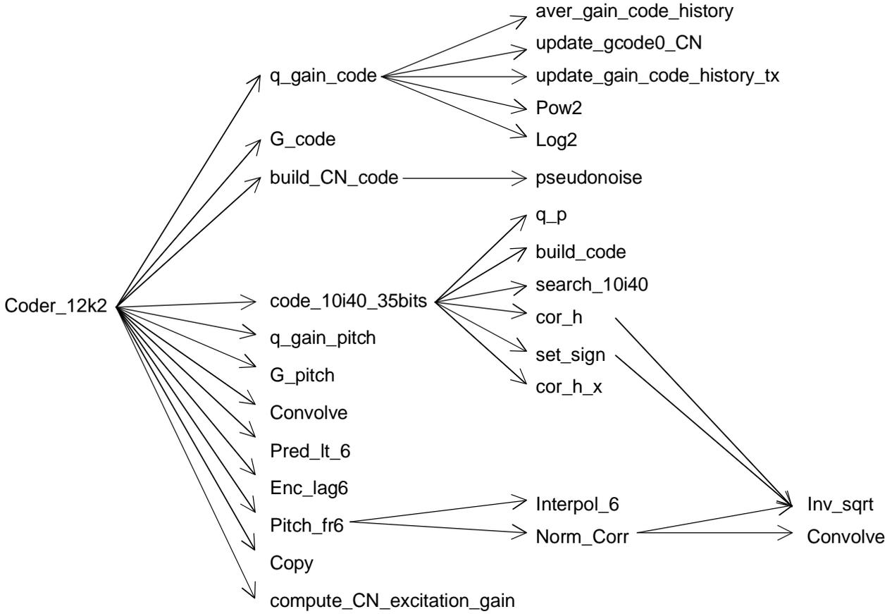
Figure 2: Speech encoder subframe processing call graph
