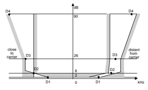
Figure B.2: IF filter characteristics
