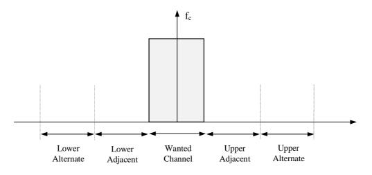
Figure 0: Adjacent and alternate channel definitions
