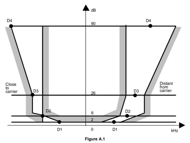
The selectivity characteristic shall keep the frequency separations shown in table A.1 from the nominal centre frequency of the adjacent channel.
