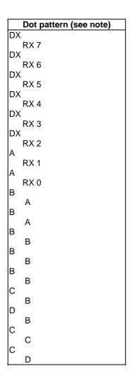
RX/DX = phasing sequence; A = Format specifier; B = Identification; C = End of sequence; D = Error check symbol;
