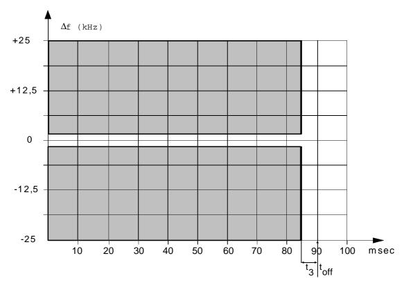
Figure 4: Switch on/off conditions
