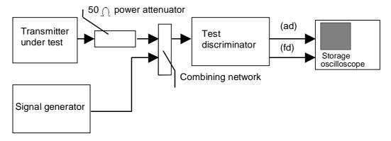
Figure 3: Measurement arrangement
