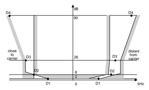
Figure D.1: IF filter characteristics
