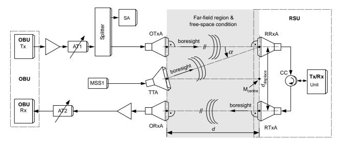
Figure B.7: RSU receive parameter measurement arrangement with CC for an EUT with a combined Rx and Tx unit / connector
