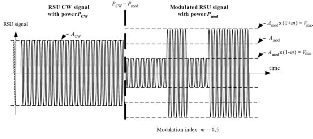
Figure B.10: RSU transmit signal
