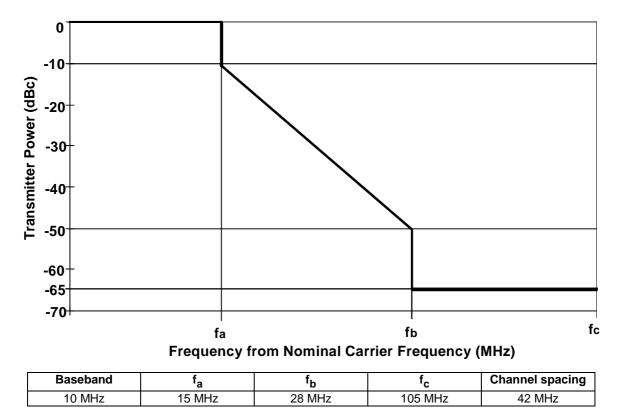
Figure 2b: Limits of spectral power density for video, wide frequency deviation
