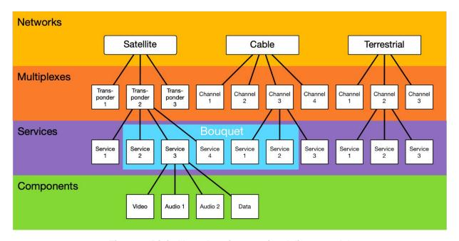
Figure 1: Digital broadcasting, service delivery model
