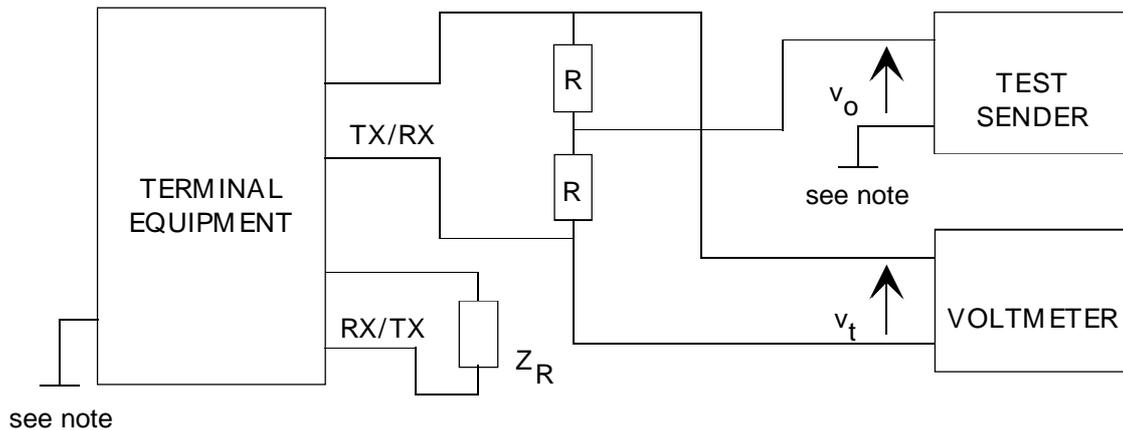
The resistors R shall be  $300 \Omega \pm 1 \%$  and matched to better than 0,1 %.
