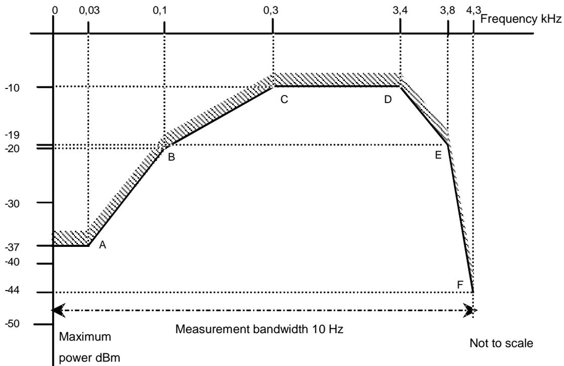
**Figure 3: Maximum power in a 10 Hz bandwidth**
