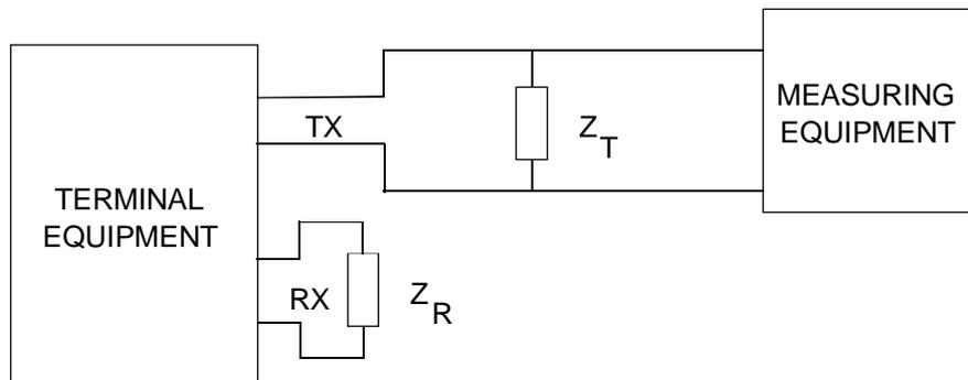
**Figure A.7: Maximum sending power above 4,3 kHz**
