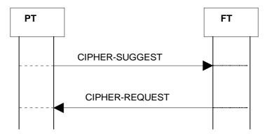
Figure 68: Ciphering, PT initiated
