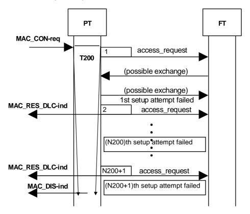
Figure 107: Bearer setup attempt fails N200+1 times
