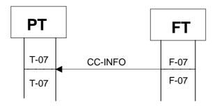
Figure 79: Call connection example, in F-07
