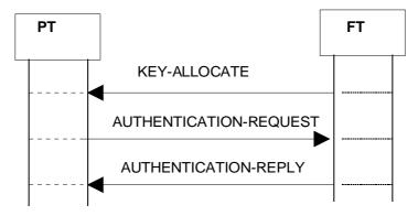
Figure 93: Authentication of FT fails
