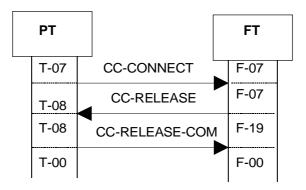
Figure 42: FT releases the incoming call transaction
