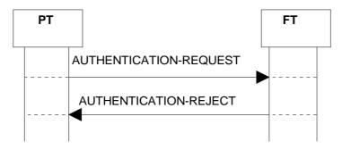
Figure 85: Authentication algorithm/key not supported by the FT
