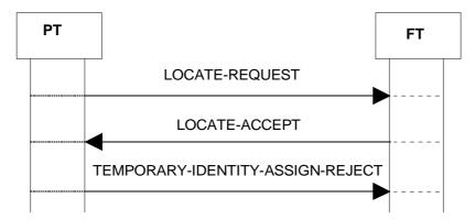
Figure 56: Rejection of identity assignment
