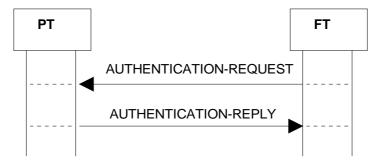
Figure 87: Authentication of PT using DSAA2
