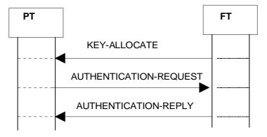
Figure 65: Authentication of FT fails
