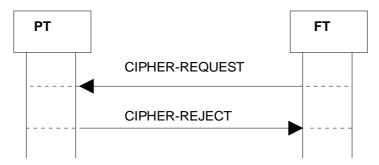
Figure 95: PT rejects the cipher request
