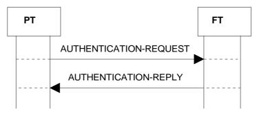
Figure 47: Authentication of FT using DSAA
