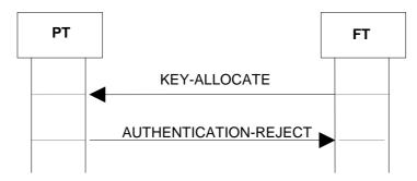
Figure 91: Allocation-type unacceptable for PT
