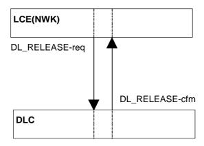
Figure 76: Link release "normal", initiating side
