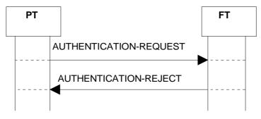
Figure 48: Authentication algorithm/key not supported by the FT
