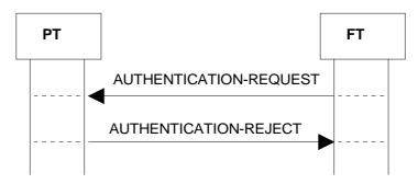
Figure 51: Authentication algorithm/key not supported by the PT
