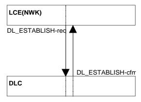
Figure 73: Direct PT initiated link establishment, initiating side
