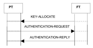
Figure 90: Key allocation using DSAA2
