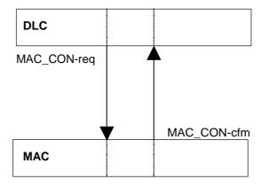
Figure 99: Establishment of a MAC connection initiating side
