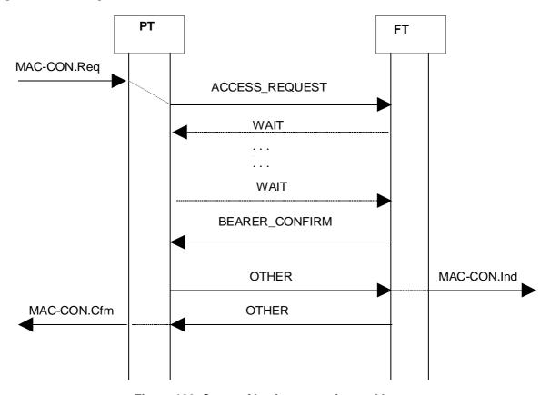
Figure 106: Setup of basic connection and bearer
