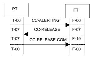
Figure 38: FT releases the incoming call transaction
