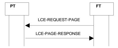
Figure 70: Indirect FT initiated link establishment
