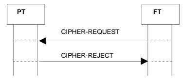
Figure 67: PT rejects the cipher request
