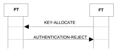
Figure 63: Allocation-type unacceptable for PT
