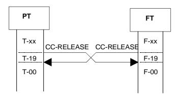
Figure 23: Both sides send {CC-RELEASE}
