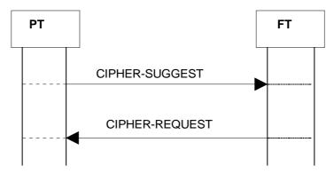
Figure 96: Ciphering, PT initiated
