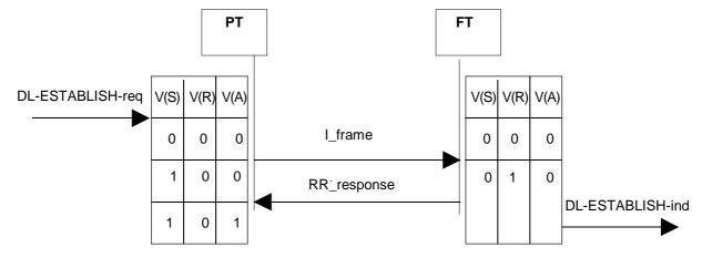
Figure 98: Class A link establishment
