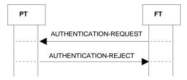
Figure 88: Authentication algorithm/key not supported by the PT
