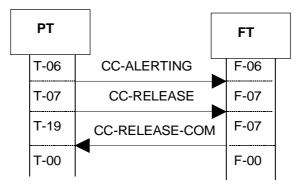
Figure 39: PT release the incoming call transaction
