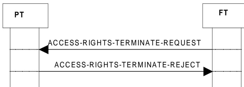
**Figure 60: PT rejects****Table 55: Standard values used within the {ACCESS-RIGHTS-TERMINATE-REJECT} message**
