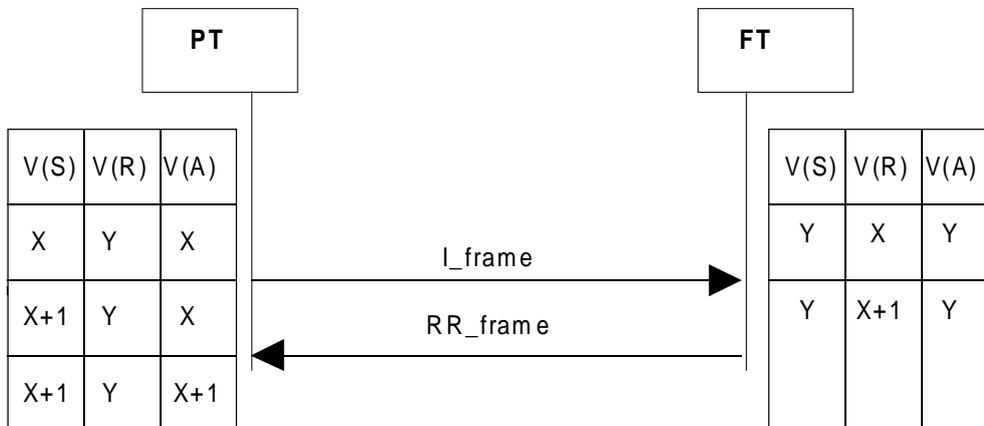
NOTE 1: During the calculation of the variable's values an assumption has been made that the I\_frame sent by PT is not used for acknowledgement of previous received I\_frames and is not a re-transmission.
