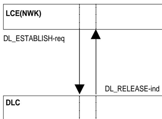
Figure 74: Direct PT initiated link establishment failure
