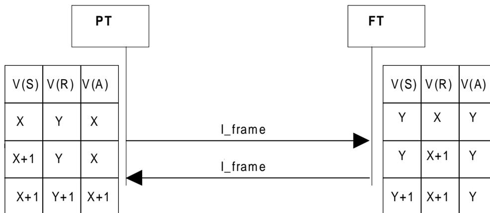
NOTE 1: During the calculation of the variable's values the assumptions have been made that the I\_frame sent by PT is not used for acknowledgement of previous received I\_frames and, both frames are not re-transmission.
