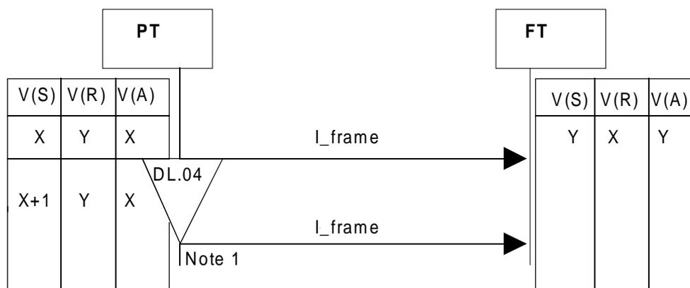
NOTE 1: The I\_frame is re-transmitted only if  $N250 < \text{max.value}$ .
