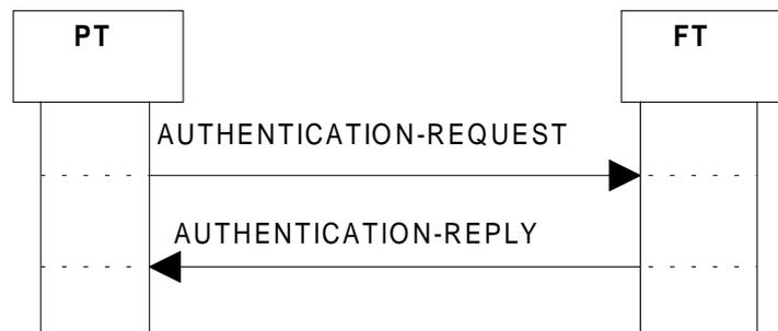
NOTE: If the received RES value in the {AUTHENTICATION REPLY} message is not equal to XRES1 further actions taken by the PT depend on the PP application.
