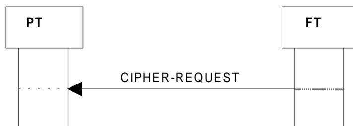
**Figure 65: Cipher - switching initiated by FT**
