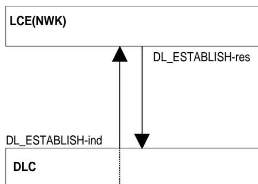
Figure 73: Direct PT initiated link establishment, receiving side
