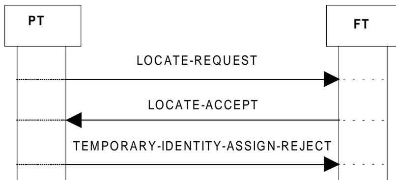
**Figure 55: Rejection of identity assignment****Table 48: Values used within the {TEMPORARY-IDENTITY-ASSIGN-REJECT} message**
