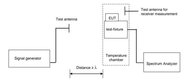
Figure 6: Validation of test set-up with EUT in place
