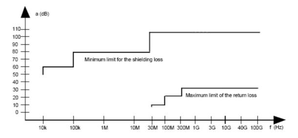
Figure E.3: Specification for shielding and reflections
