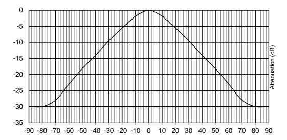
Figure I.7: Minimum attenuation of the vertical antenna pattern
