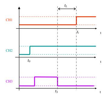
Figure I.3: Minimum listen time after detection,  $t_I$ , measurement
