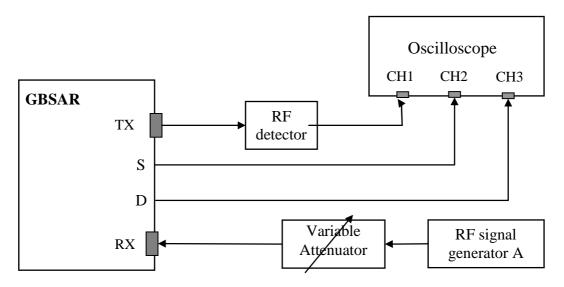
Figure I.1: DAA measurement arrangement
