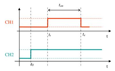
Figure I.4: Maximum transmit on-time,  $t_{on}$ , measurement
