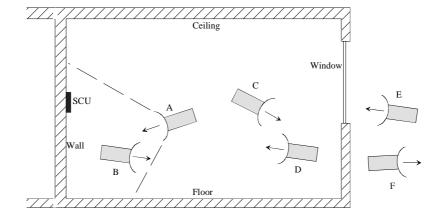
Figure H.1: Example for RFID system with an automatic RF power control for in- and outside building operation
