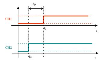
Figure I.2: Minimum listen time,  $t_D$ , measurement
