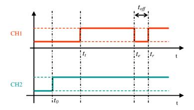
Figure I.5: Maximum transmit off-time,  $t_{\it off}$ , measurement
