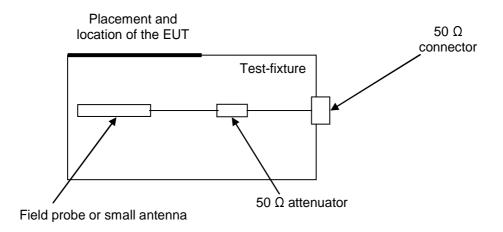
Figure 4: Test fixture
