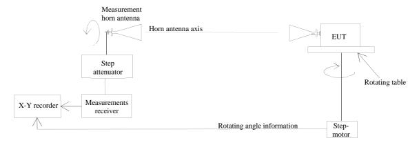
Figure I.6: Test set-up for measurement of antenna pattern
