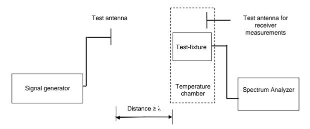
Figure 5: Validation of test set-up without EUT
