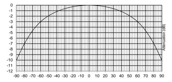
Figure I.8: Minimum attenuation of the horizontal antenna pattern
