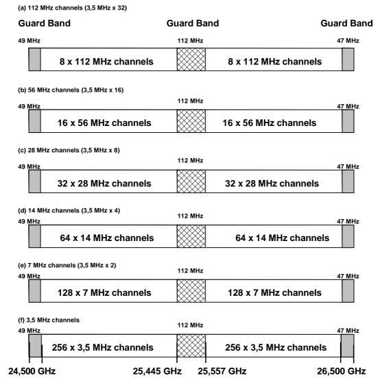
Figure A.1: Radio frequency channel arrangement
