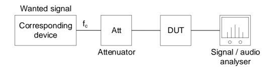
Figure 9: Receiver sensitivity test setup
