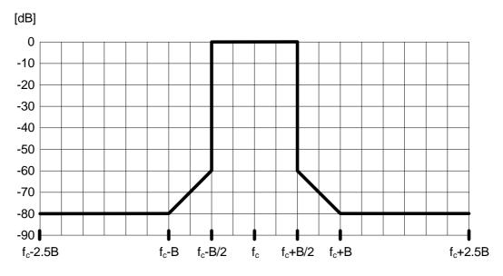
Figure 1: Transmit spectral power mask for equipment employing analogue modulation, RBW = 1 kHz
