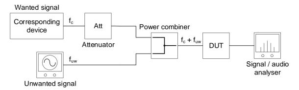
Figure 10: Test setup for receiver adjacent channel selectivity
