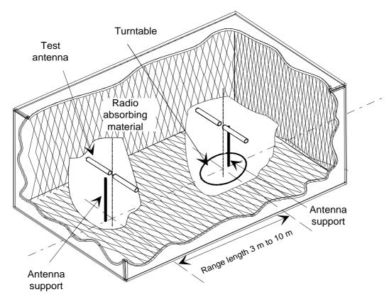
Figure D.1: A typical anechoic chamber
