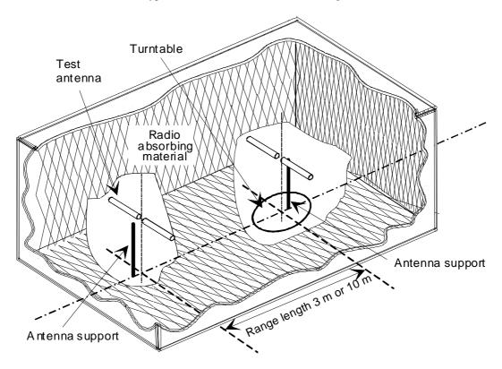
Figure A.1: A typical Anechoic Chamber
