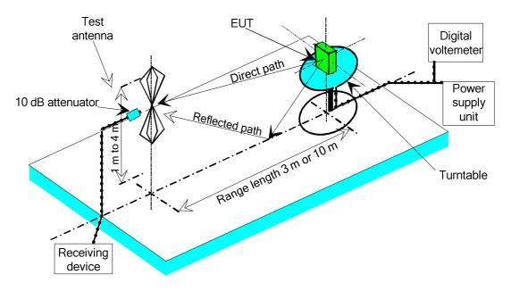
Figure A.4: Measuring arrangement on ground plane test site (OATS set-up for spurious emission testing)
