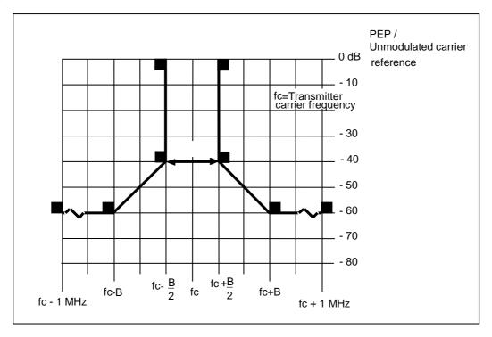
Figure 5: Spectrum mask for digital systems above 2 GHz
