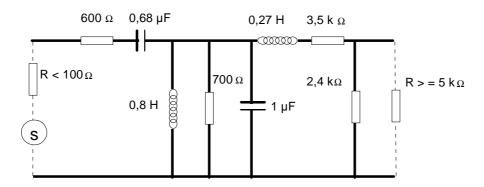
Figure 2: Filter circuit
