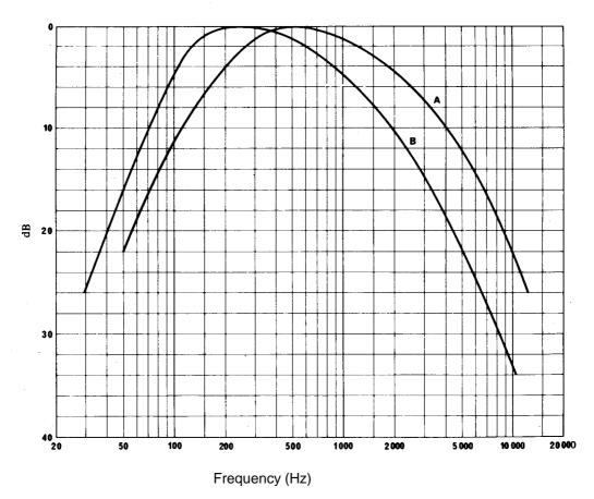
NOTE 1: Curve A = Frequency spectrum of standardized noise (measured with one-third octave filters). NOTE 2: Curve B = Frequency response characteristics of filter circuit.
