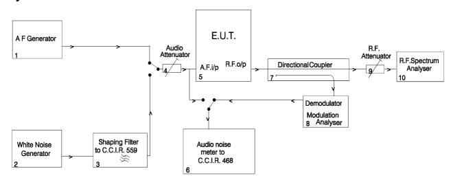
NOTE: If the EUT incorporates ancillary coding or signalling channels, for example, pilot tone, etc. these should be switched on prior to measuring the transmitter RF output spectrum.
