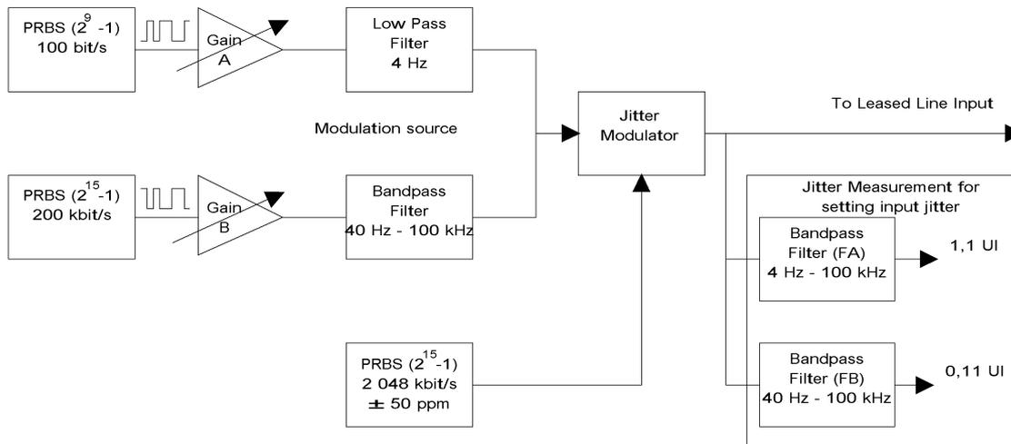
NOTE: The filter gains to determine the jitter levels are set individually. Filter FA is used when setting the value of A, with signal B disconnected. Filter FB is used when setting the value of B, with signal A disconnected.
