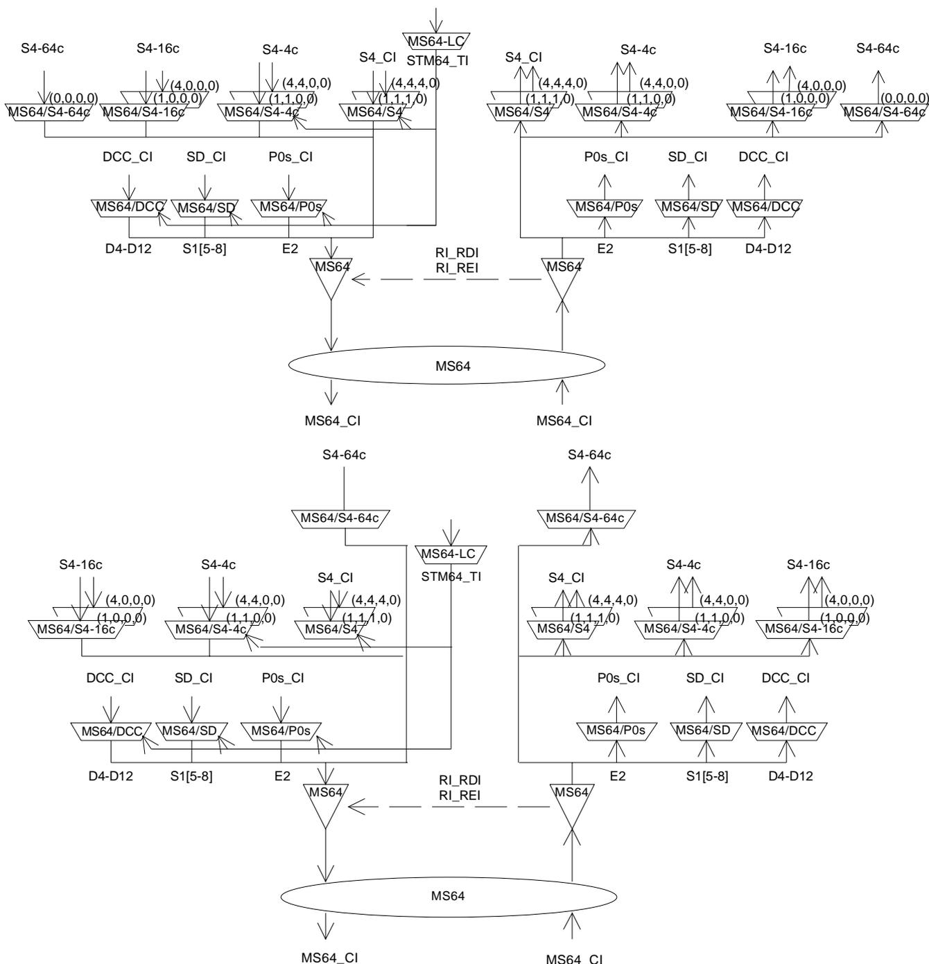
**Figure 147: STM-64 Multiplex Section atomic functions**
