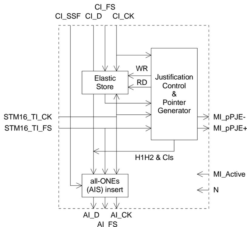
**Figure 100: Main processes within MS16/S4-4c\_A\_So**
