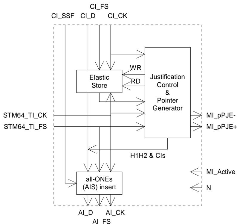
**Figure 161: Main processes within MS64/S4-16c\_A\_So**
