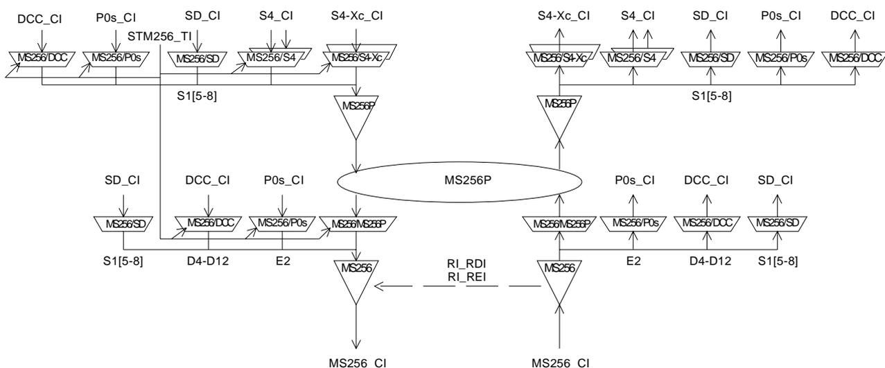
Figure 202: STM-256 Multiplex Section Linear Trail Protection Functions
