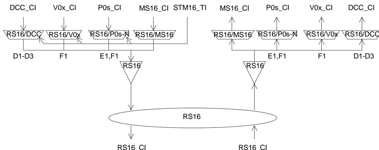
Figure 73: STM-16 Regenerator Section atomic functions
