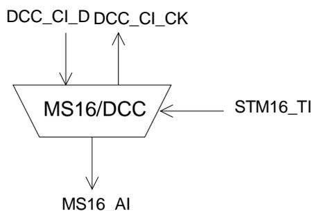
Figure 105: MS16/DCC\_A\_So symbol
