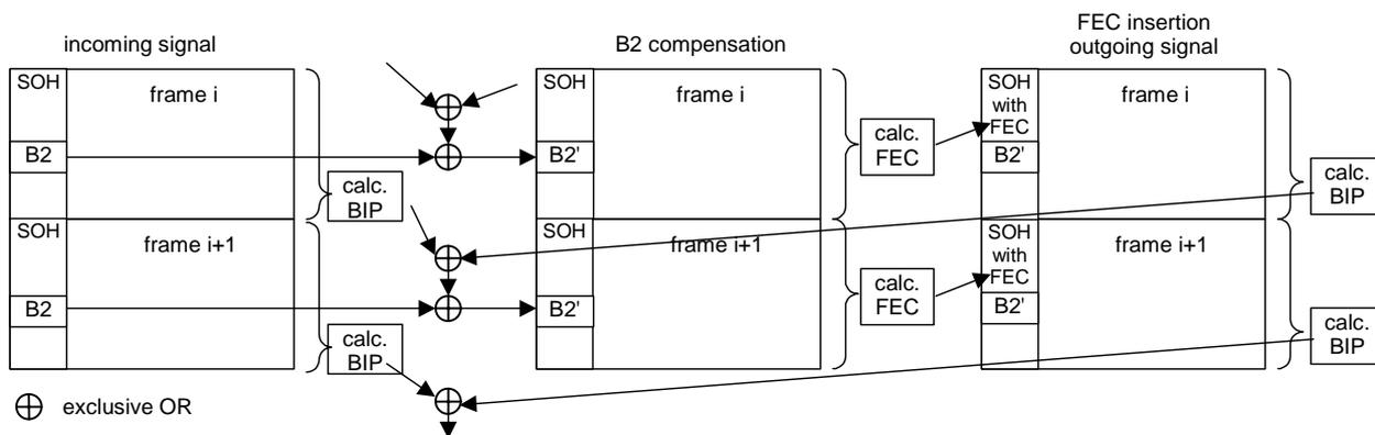
**Figure 143: B2 compensation and FEC calculation**
