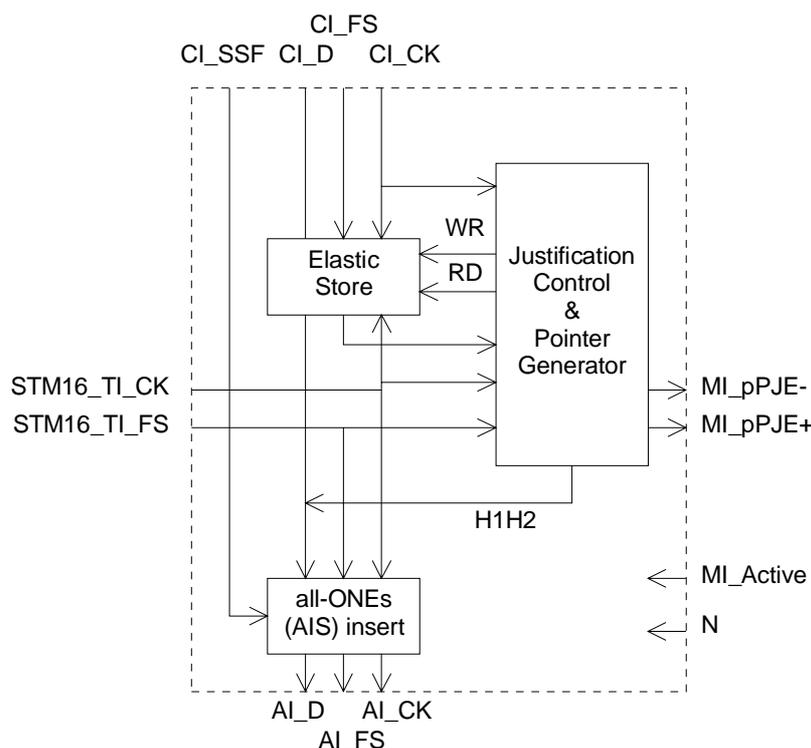
Figure 97: Main processes within MS16/S4\_A\_So
