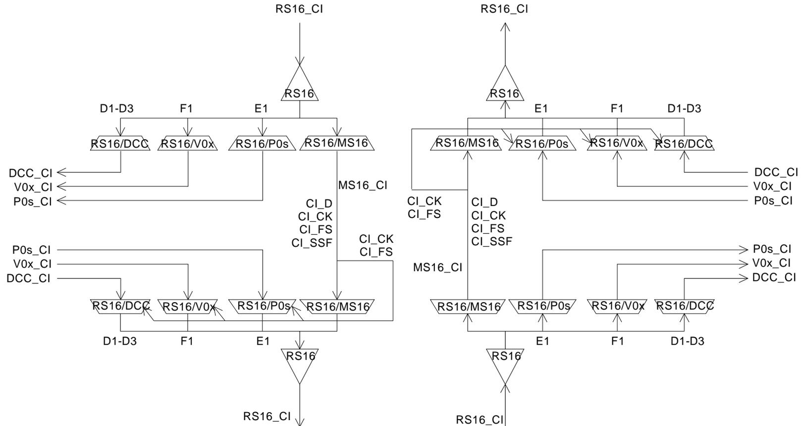
Figure B.1: STM-16 regenerator model (supporting DCC, OW, USR)
