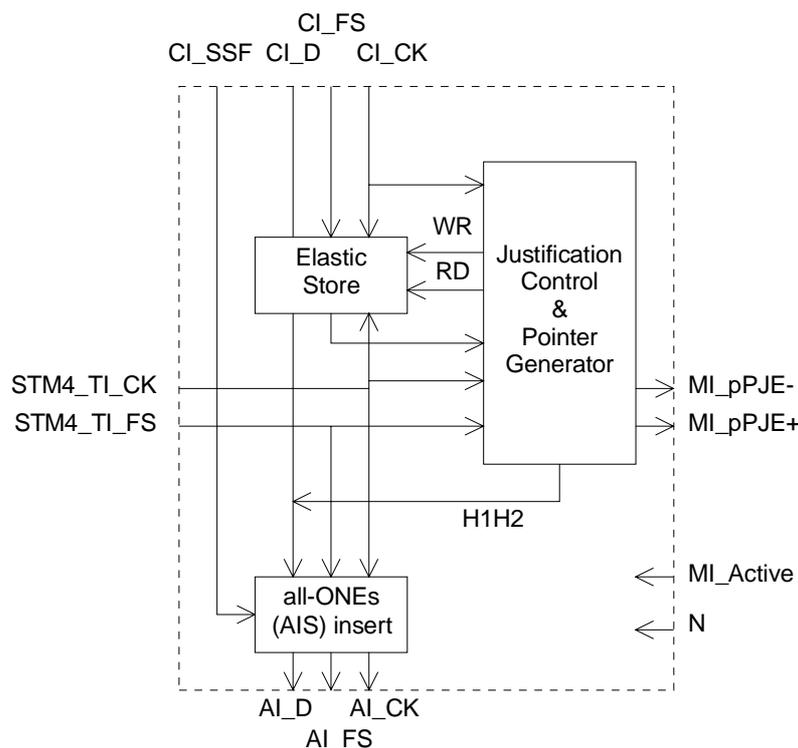
Figure 58: Main processes within MS4/S4\_A\_So
