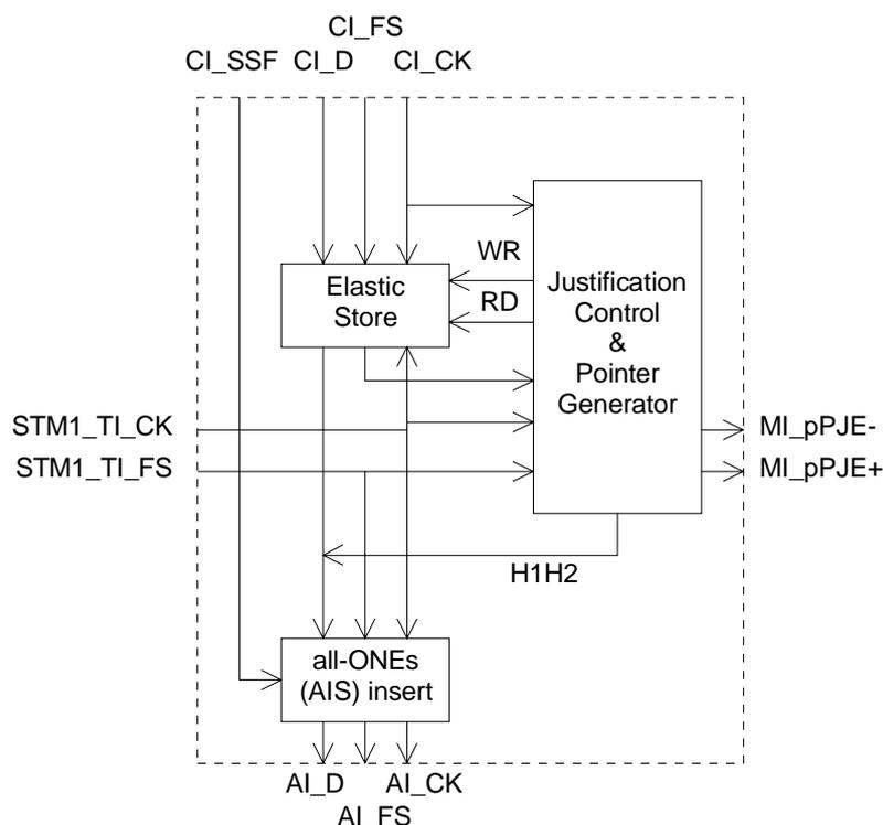
**Figure 23: Main processes within MS1/S4\_A\_So**
