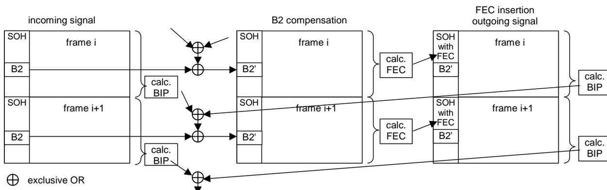
**Figure 195: B2 compensation and FEC calculation**
