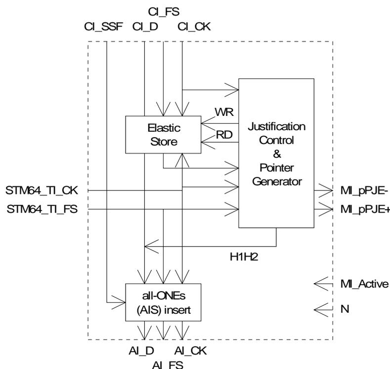
Figure 155: Main processes within MS64/S4\_A\_So
