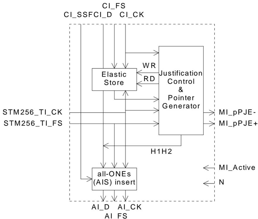
Figure 207: Main processes within MS256/S4\_A\_So
