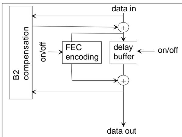
**Figure 142: STM-64 FEC encoding process**
