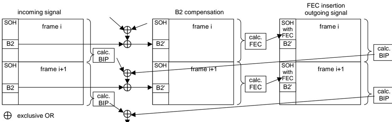
**Figure E.5: B2 compensation and FEC calculation**
