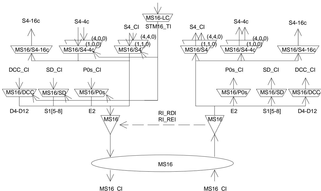
**Figure 88: STM-16 Multiplex Section atomic functions**
