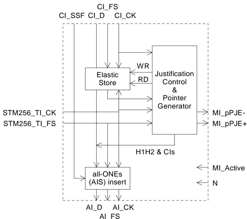
**Figure 210: Main processes within MS256/S4-4c\_A\_So**
