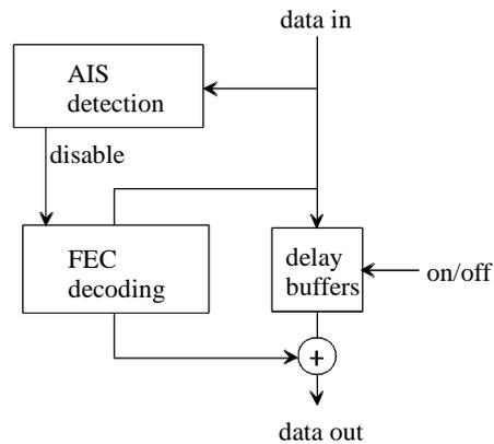
**Figure 198: STM-256 FEC decoding process**
