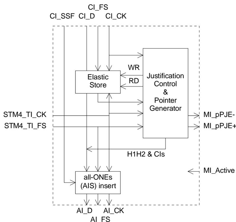
**Figure 61: Main processes within MS4/S4-4c\_A\_So**
