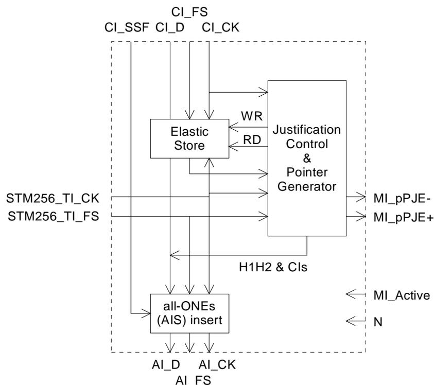
**Figure 213: Main processes within MS256/S4-16c\_A\_So**
