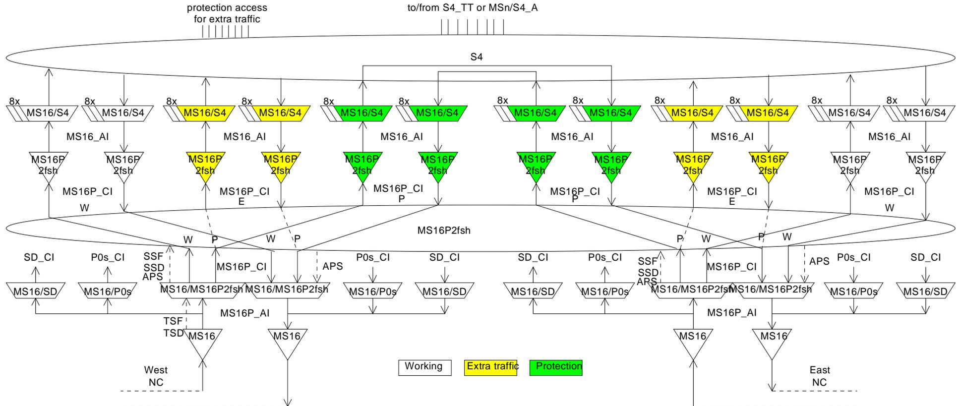
Figure 93: STM-16 Multiplex Section 2 fibre Shared Protection Ring model (working: AU-4 #1 to AU-4 #8, protection: AU-4 #9 to AU-4 #16)
