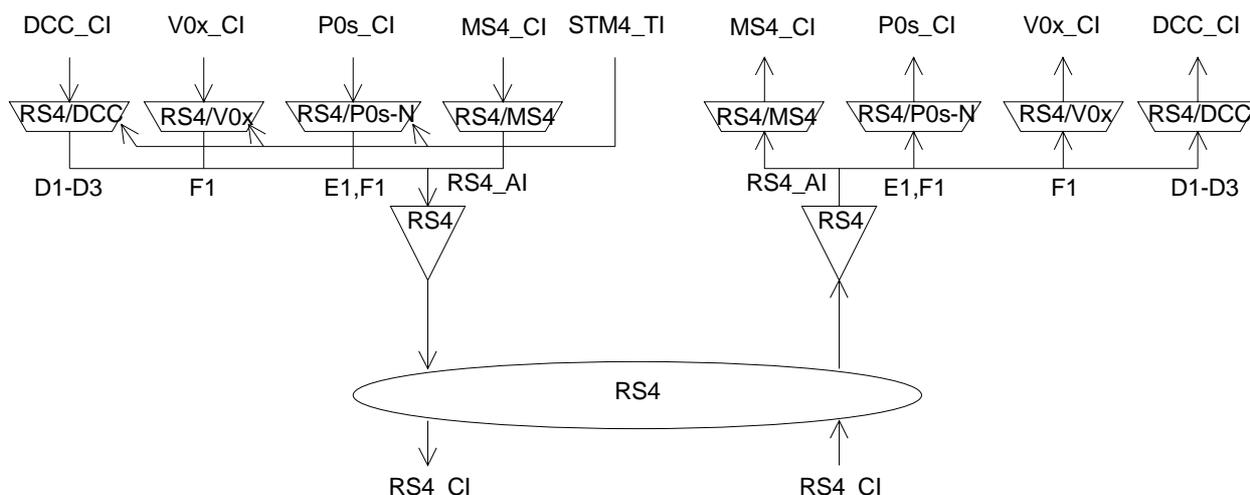
Figure 35: STM-4 Regenerator Section atomic functions
