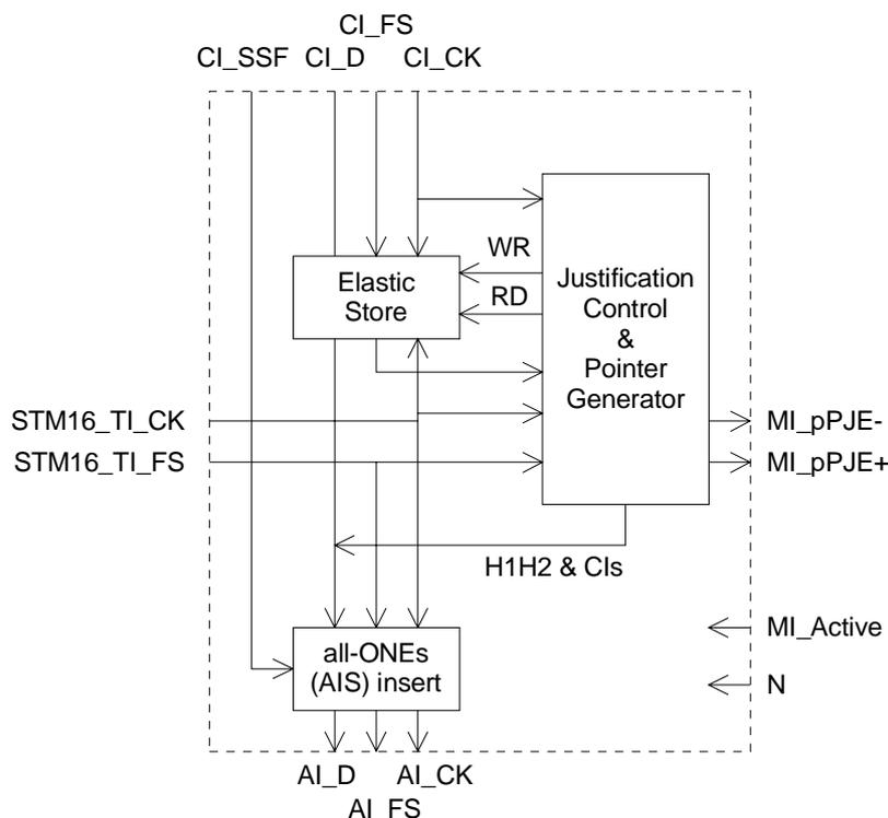
**Figure 103: Main processes within MS16/S4-16c\_A\_So**
