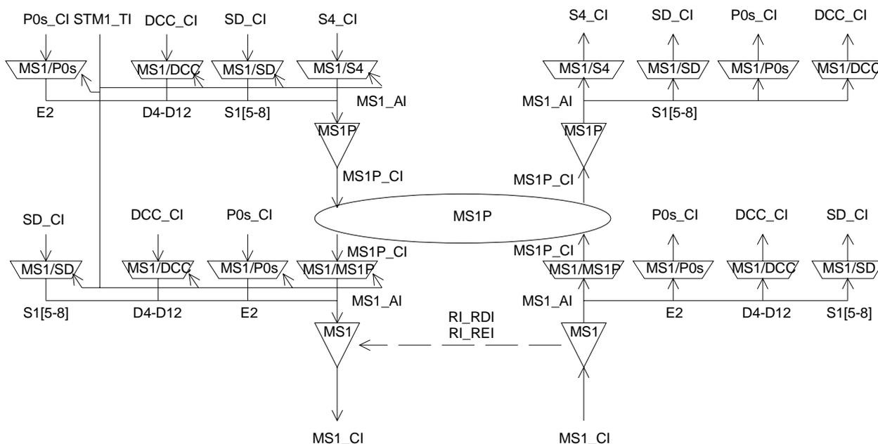
**Figure 18: STM-1 Multiplex Section Linear Trail Protection Functions**
