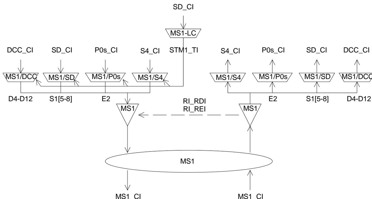
**Figure 15: STM-1 Multiplex Section atomic functions**
