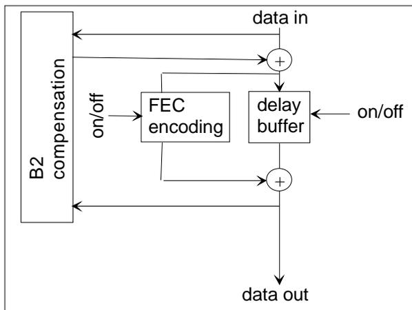
**Figure E.4: STM-16 FEC encoding process**
