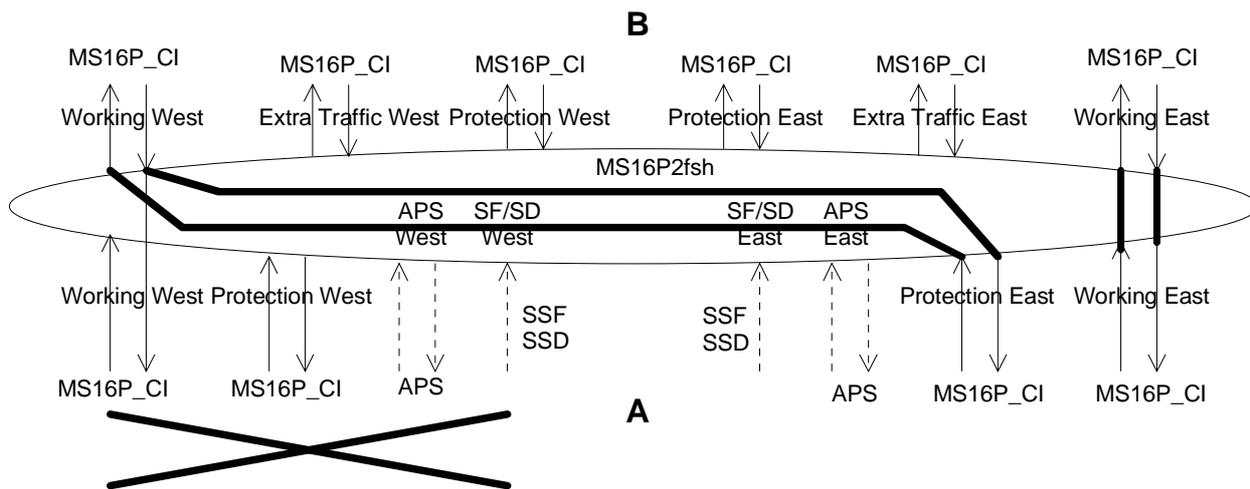
**Figure 119: Matrix connections in a network element adjacent to a fault on its west side**
