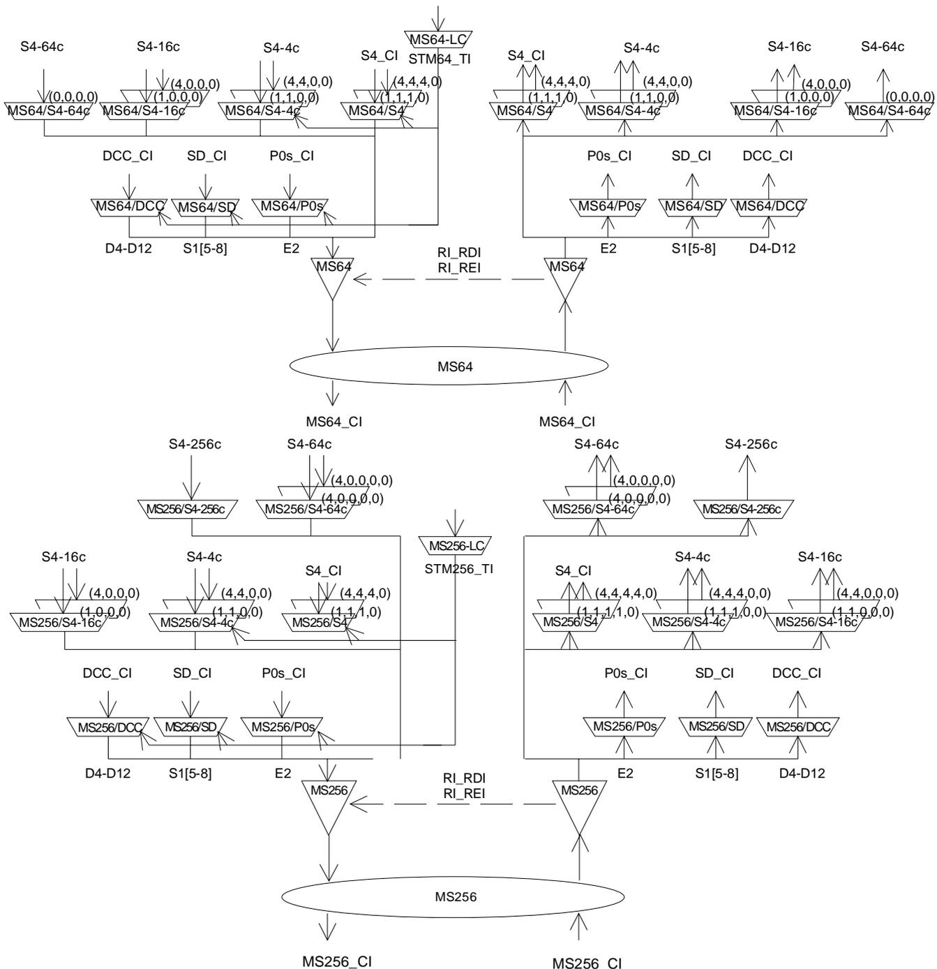
**Figure 199: STM-256 Multiplex Section atomic functions**
