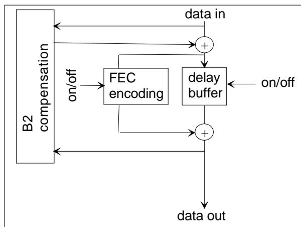
**Figure 194: STM-256 FEC encoding process**
