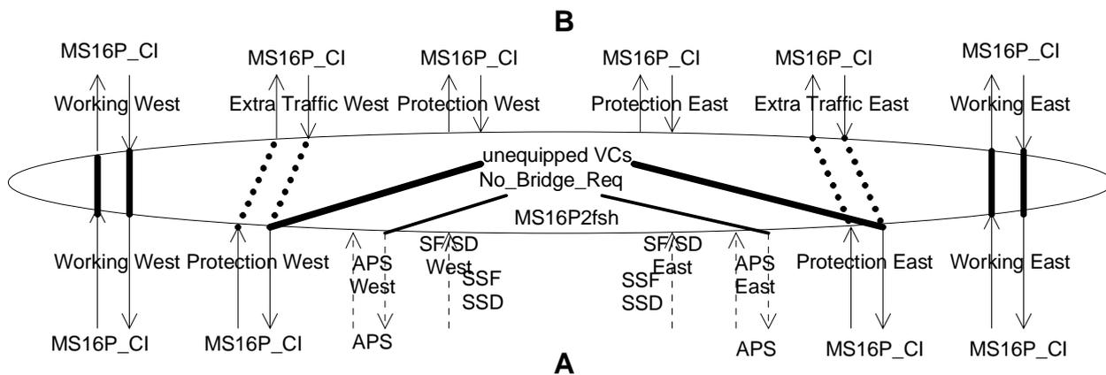
**Figure 116: Matrix connections in a network element within a ring without a fault; dotted lines represent the case of extra traffic support**
