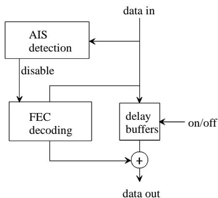
**Figure E.8: STM-16 FEC decoding process**
