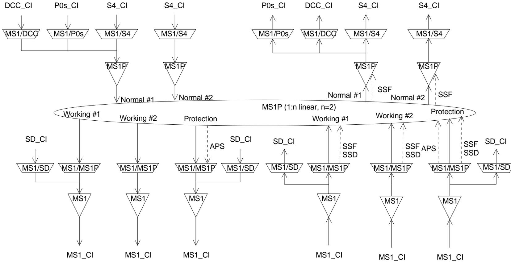
**Figure D.2: 1:n STM-1 Multiplex Section Linear Trail Protection model (Working / Normal #1 supports (protected) OW,DCC and (unprotected) SSM: Working / Normal #2 does not support OW,DCC,SSM)**
