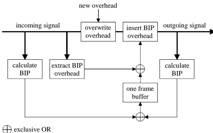
**Figure E.6: B2 correction; processes**
