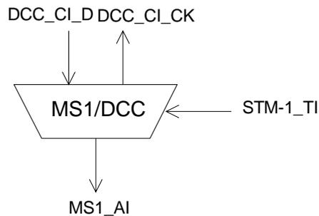
**Figure 25: MS1/DCC\_A\_So symbol**
