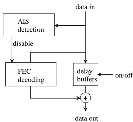
**Figure 146: STM-64 FEC decoding process**
