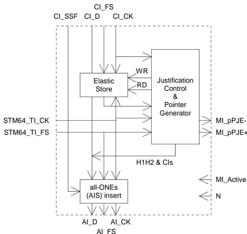
Figure 164: Main processes within MS64/S4-64c\_A\_So
