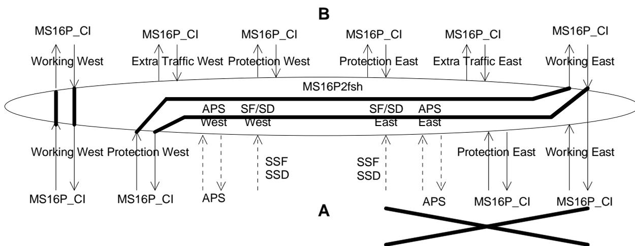
**Figure 118: Matrix connections in a network element adjacent to a fault on its East side**
