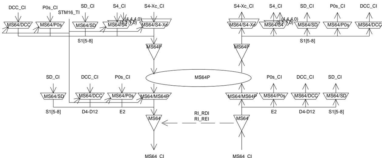
Figure 150: STM-64 Multiplex Section Linear Trail Protection Functions
