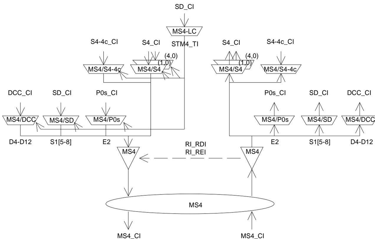
Figure 50: STM-4 Multiplex Section atomic functions
