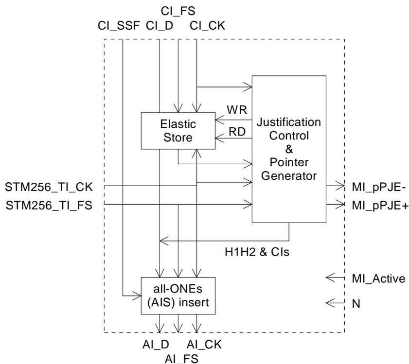
**Figure 219: Main processes within MS256/S4-256c\_A\_So**
