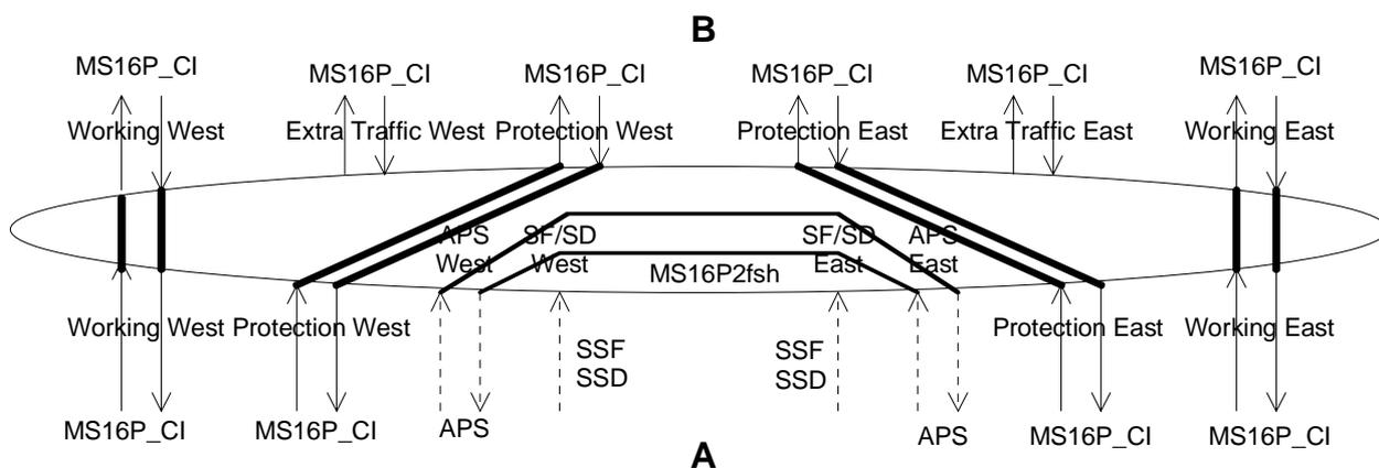
**Figure 117: Matrix connections in a network element not adjacent to a fault**
