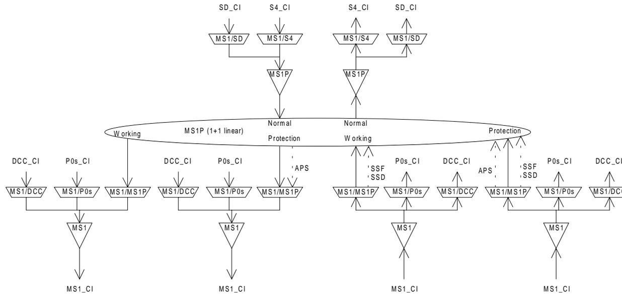
**Figure D.1: 1+1 STM-1 Multiplex Section Linear Trail Protection model
