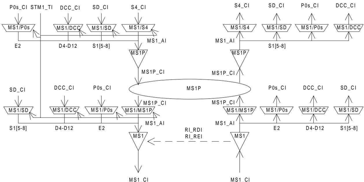
**Figure 19: STM-1 Multiplex Section Linear Trail Protection Functions**
