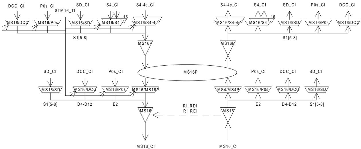
Figure 92: STM-16 Multiplex Section Linear Trail Protection Functions
