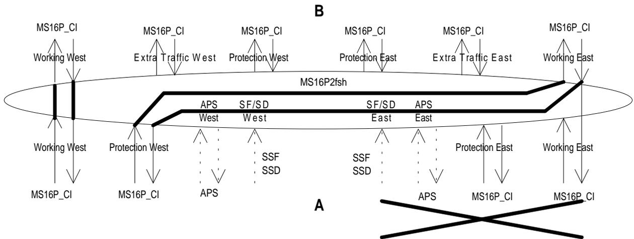
**Figure 116: Matrix connections in a network element adjacent to a fault on its East side**
