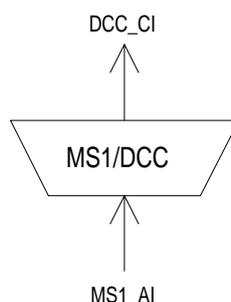
Figure 27: MS1/DCC\_A\_Sk symbol
