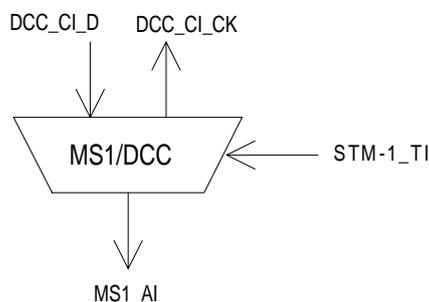
Figure 26: MS1/DCC\_A\_So symbol
