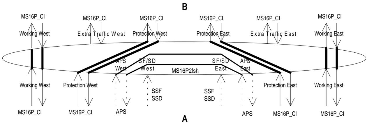
**Figure 115: Matrix connections in a network element not adjacent to a fault**
