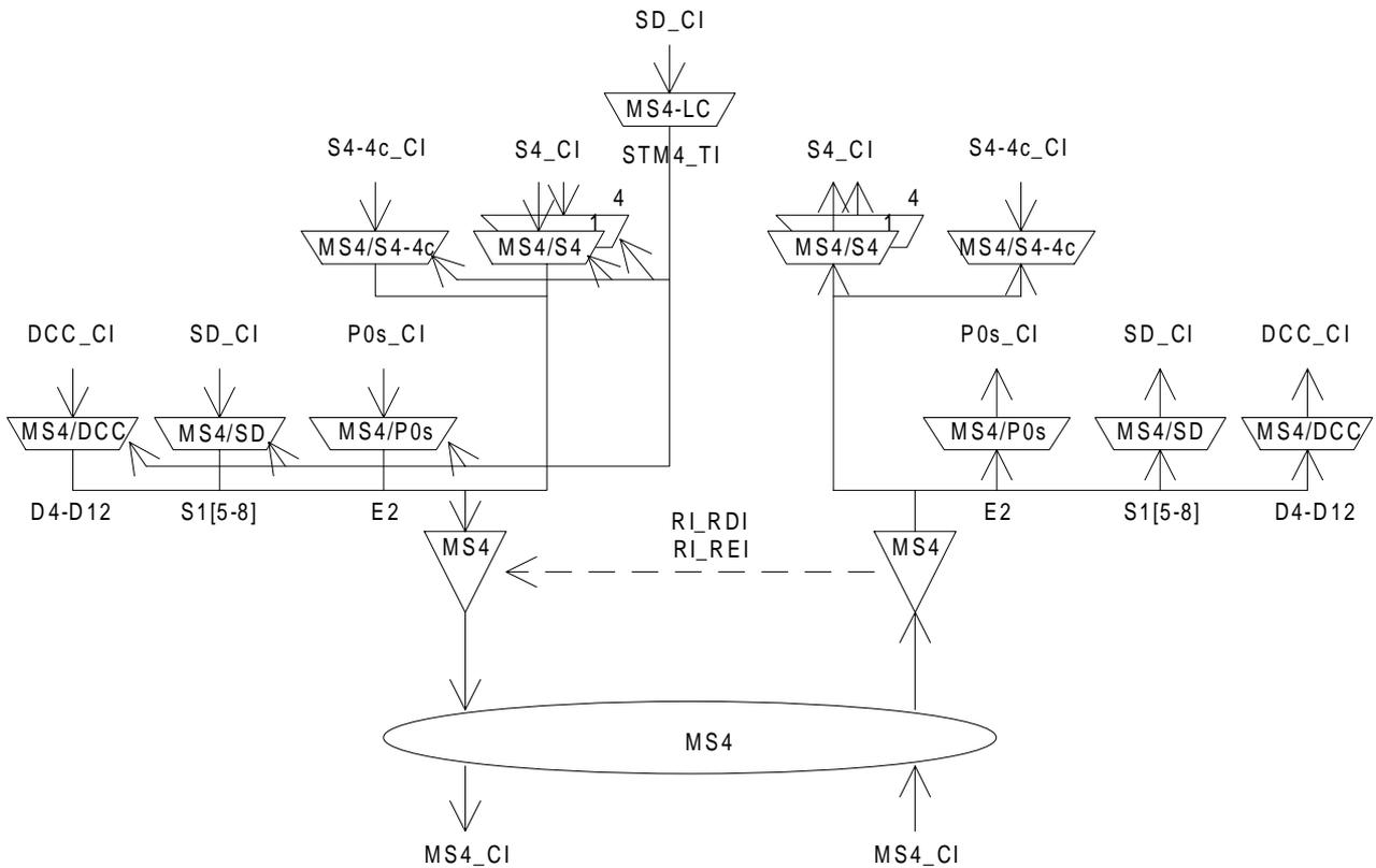
Figure 51: STM-4 Multiplex Section atomic functions
