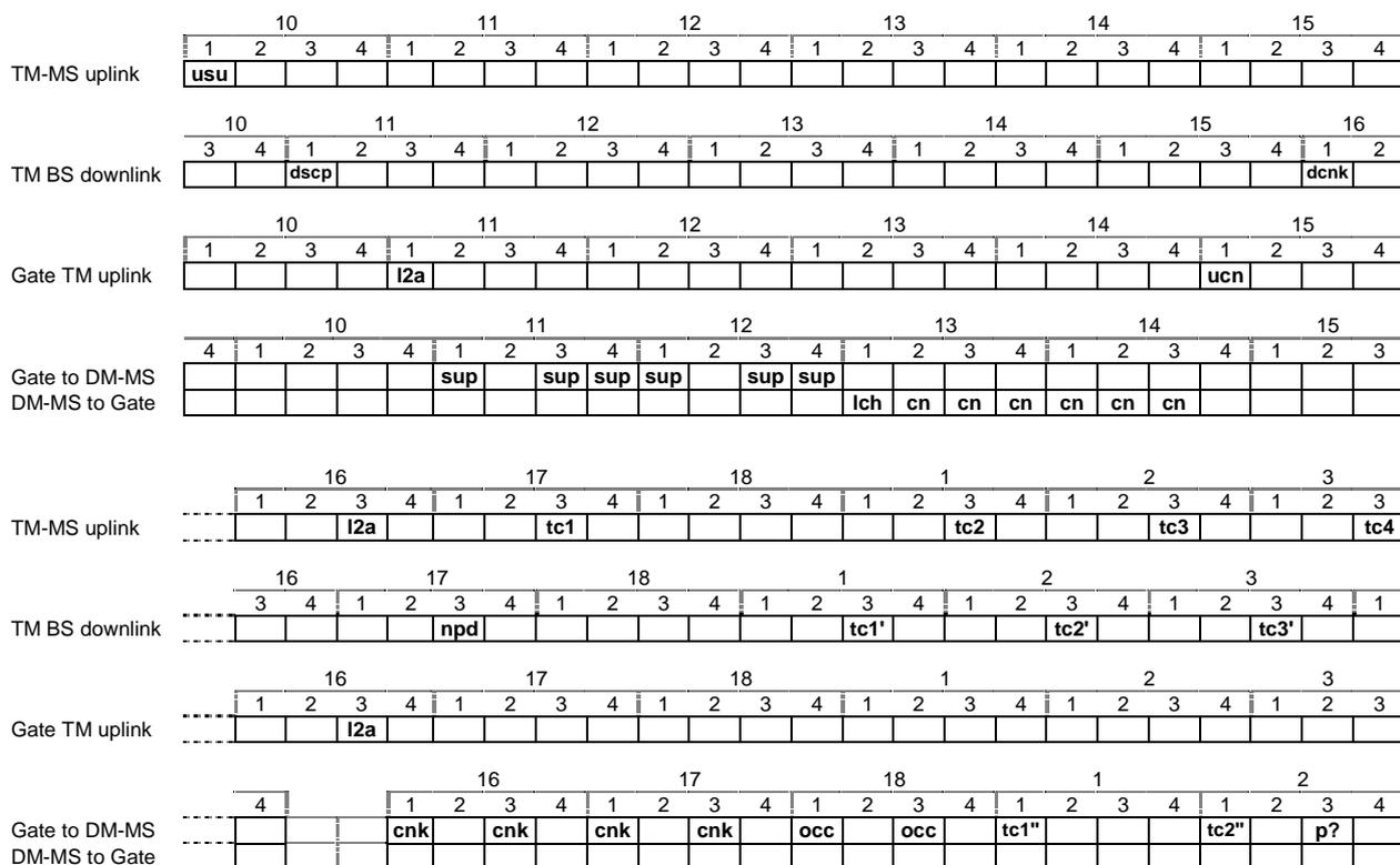
**Figure 7: Timing diagram for individual call from TM-MS via DM-GATE**
