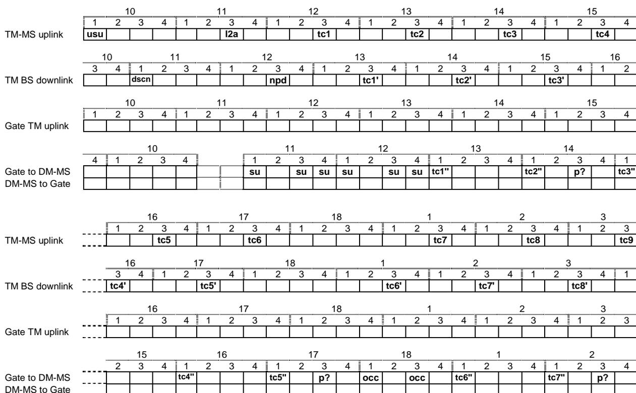
Figure 3: Timing diagram for group call from TMO via DM-GATE
