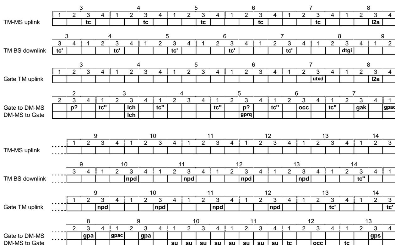
Figure 13: Timing diagram for pre-emption of a call through a DM-GATE
