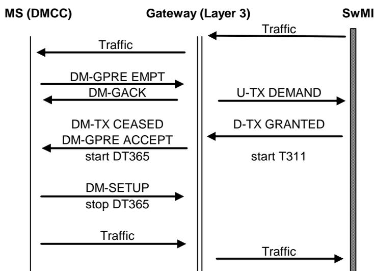
**Figure 24: DM-MS pre-emption for continuation of ongoing call**
