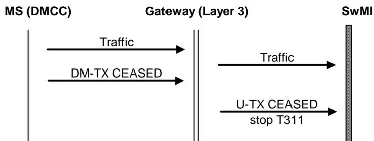
Figure 20: End of traffic transmission by master DM-MS
