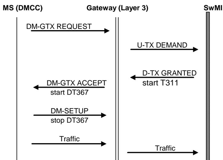
Figure 21: DM transmit request during DM channel reservation
