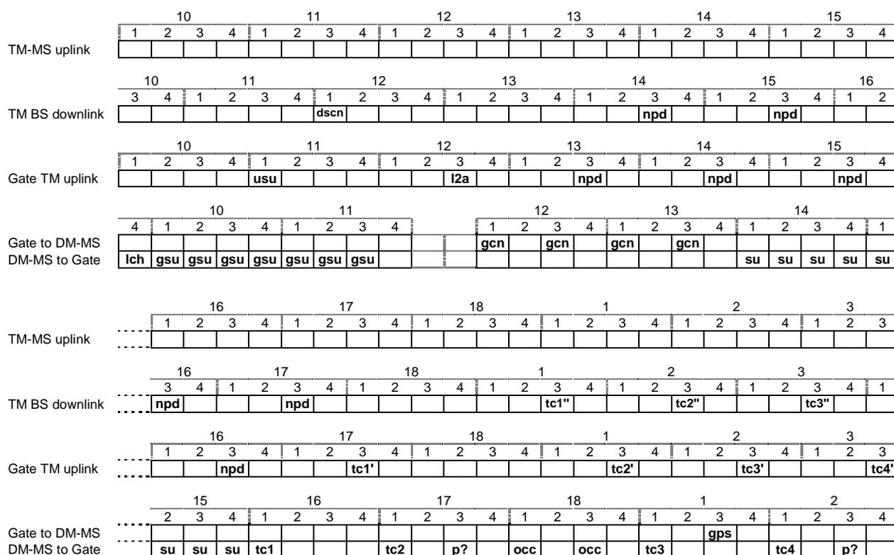
**Figure 5: Timing diagram for group call from DM-MS via DM-GATE**
