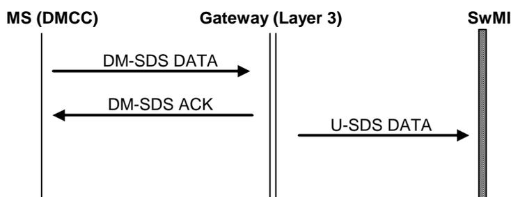
**Figure 28: Outgoing DM SDS message to TMO**
