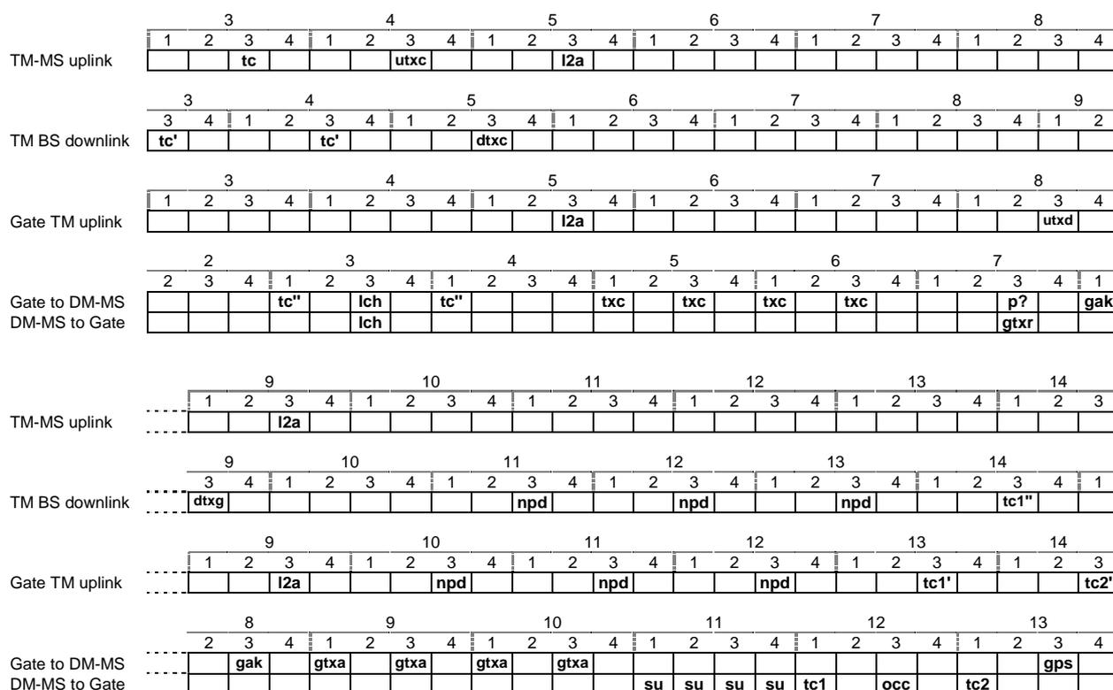
Figure 11: Timing diagram for a changeover of an individual call from TM-MS to DM-MS
