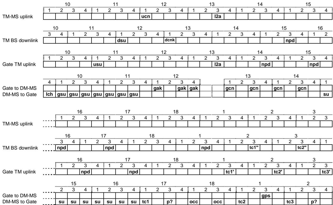
Figure 9: Timing diagram for individual call from DM-MS to TM-MS via DM-GATE
