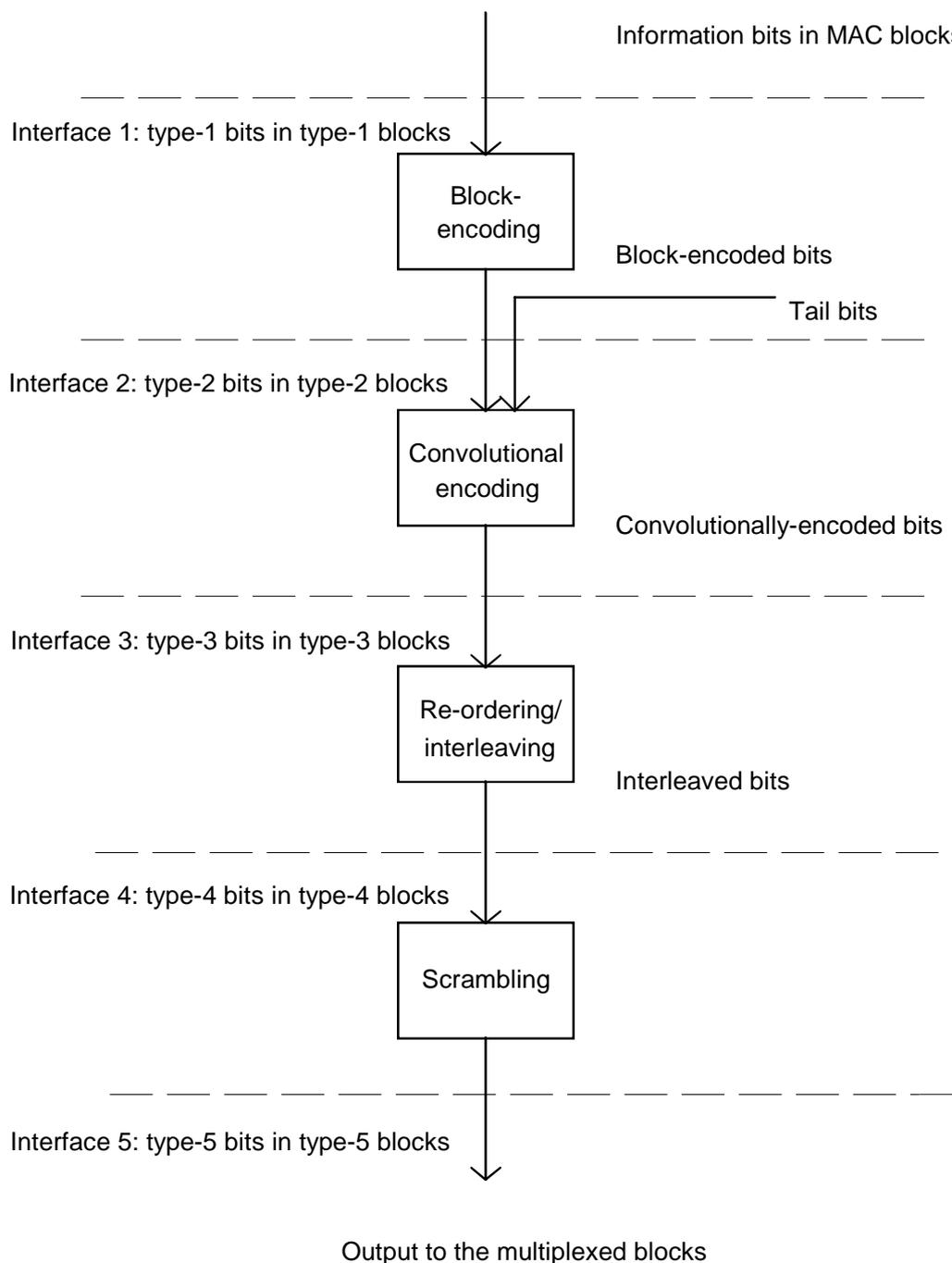
**Figure 6: Interfaces in the error control structure**
