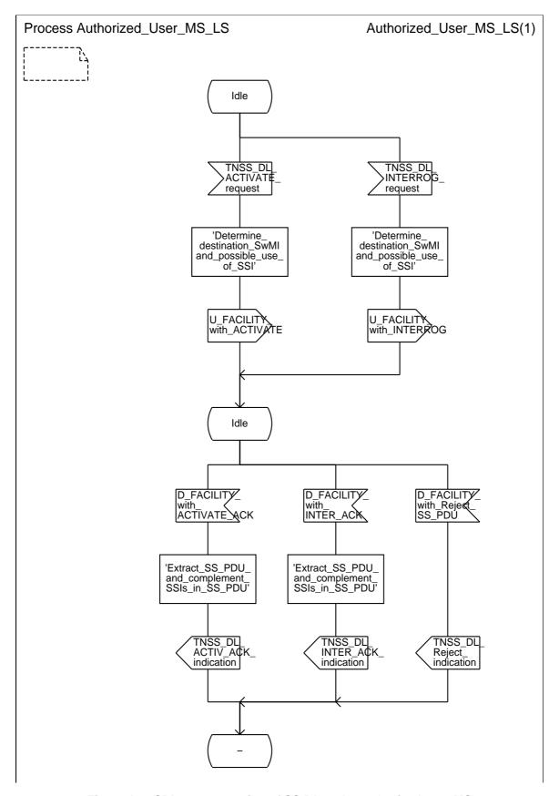
Figure A.4: SDL representation of SS-DL at the authorized user MS
