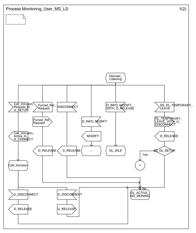
Figure A.1 (sheet 2 of 2): Monitoring user MS SDL
